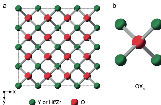
Fig. 5 (a) Structure of a typical  $\text{A}_2\text{B}_2\text{O}_7$  defect fluorite material. Red spheres denote O sites (1/8 of which will be vacant) and green spheres the single cation site. (b) Expansion showing the oxygen coordination environment, where the cation sites can be occupied either by A or B cations.
