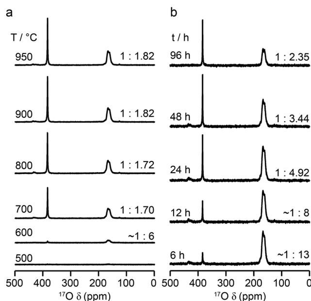
Fig. 3  $^{17}\text{O}$  (14 T, 21 kHz) MAS NMR spectra of  $\text{Y}_2\text{Sn}_2\text{O}_7$  enriched (a) for 12 h at the temperatures shown and (b) at 600 °C for the durations shown. Spectra were acquired using the same mass of sample and by averaging the same number of transients (note that the two spectra enriched at 600 °C are from different samples and the error on this measurement is greater owing to the low level of enrichment).
