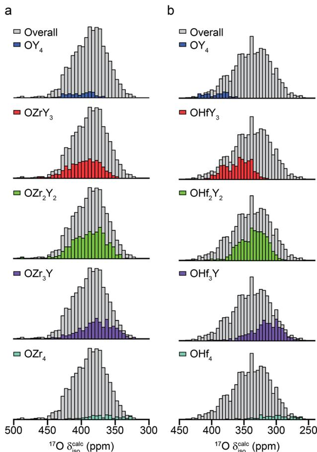
Fig. 7 Calculated  $^{17}O$  chemical shifts for  $\sim 30$  structural models of (a)  $Y_2Zr_2O_7$  and (b)  $Y_2Hf_2O_7$ , separated by local atomic environment. Points corresponding to the four additional pyrochlore-based structural models (described in detail in the ESI (S10†)) are not included.
