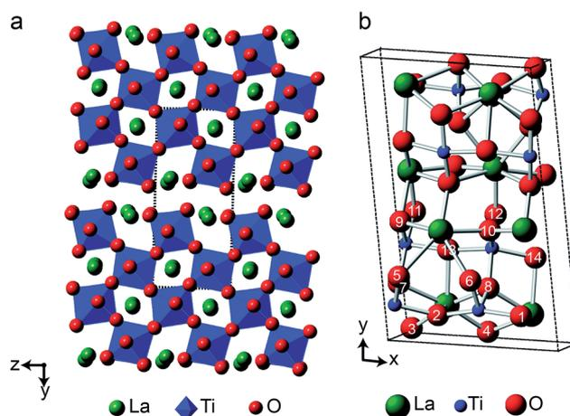
Fig. 8 (a) Structure of layered perovskite  $La_2Ti_2O_7$ , viewed down the (100) axis. Red spheres denote O, green spheres denote La cations, and  $TiO_6$  octahedra are shown in blue. The dashed lines indicate the monoclinic unit cell. (b) Monoclinic unit cell of  $La_2Ti_2O_7$  viewed down the (001) axis, with the crystallographically distinct O species indicated.
