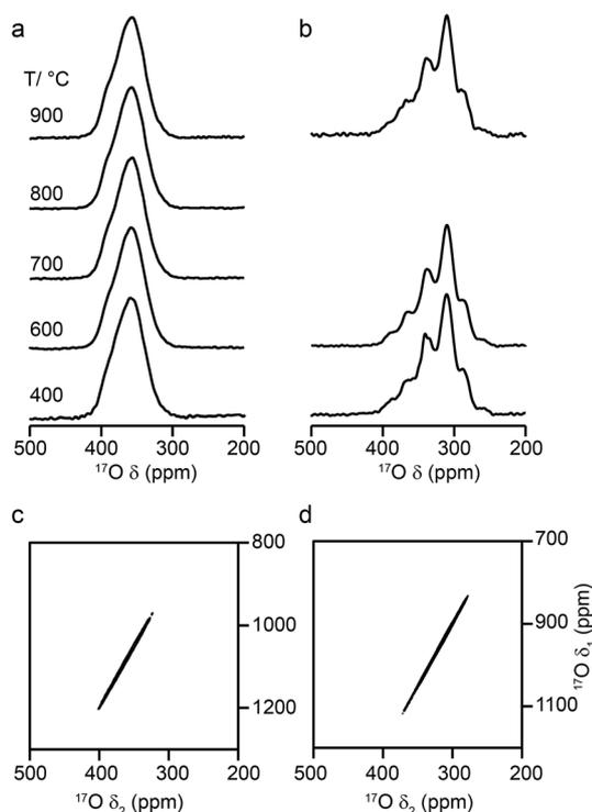
Fig. 6  $^{17}\text{O}$  (14.1 T, 21 kHz) MAS NMR spectra of (a)  $\text{Y}_2\text{Zr}_2\text{O}_7$  and (b)  $\text{Y}_2\text{Hf}_2\text{O}_7$  enriched at temperatures between 400 and 900 °C for 24 h. (c, d)  $^{17}\text{O}$  (20.0 T, 21 kHz) triple-quantum MAS NMR spectra, acquired using a z-filtered pulse sequence, of (c)  $\text{Y}_2\text{Zr}_2\text{O}_7$  and (d)  $\text{Y}_2\text{Hf}_2\text{O}_7$  enriched at 950 °C for (c) 24 h and (d) 48 h.
