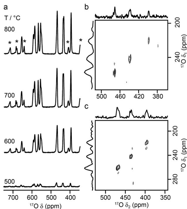
Fig. 9 (a)  $^{17}\text{O}$  (14.1 T, 21 kHz) MAS NMR spectra of  $\text{La}_2\text{Ti}_2\text{O}_7$  enriched for 12 h at temperatures between 500 and 800 °C. (b, c)  $^{17}\text{O}$  triple-quantum MAS NMR spectra, acquired using a z-filtered pulse sequence (and shown after a shearing transformation), of  $\text{La}_2\text{Ti}_2\text{O}_7$  enriched at 950 °C for 48 h, acquired at (b) 14.1 T with 20 kHz MAS and (c) 9.4 T with 13.5 kHz MAS.
