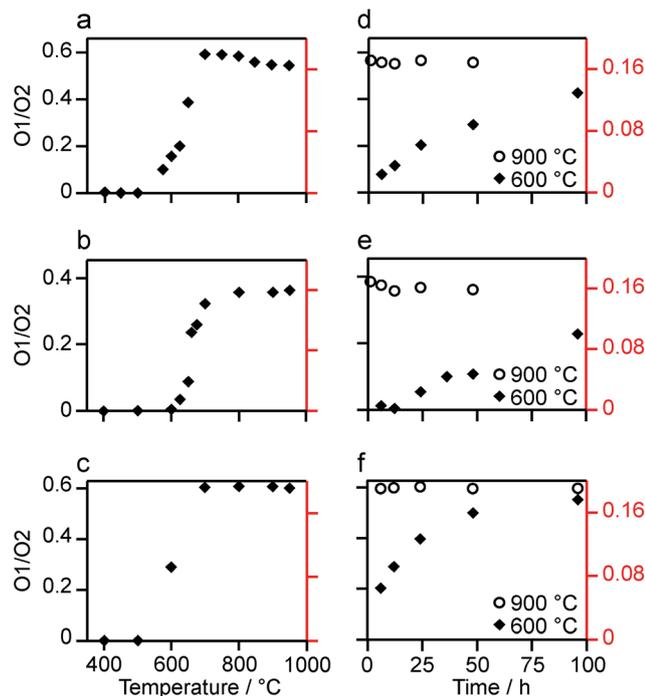
Fig. 4 Plots showing the (integrated) intensity ratio, O1/O2, extracted from  $^{17}\text{O}$  MAS NMR spectra of (a, d)  $\text{Y}_2\text{Sn}_2\text{O}_7$ , (b, e)  $\text{Y}_2\text{Ti}_2\text{O}_7$  and (c, f)  $\text{La}_2\text{Sn}_2\text{O}_7$ , enriched (a–c) for 12 h at the temperatures shown and (d–f) at 600 °C (diamonds) and 900 °C (circles) for the durations shown. Axes in red show the O1/O2 ratio corrected for the effects of relaxation and the contribution of the ST (see text).
