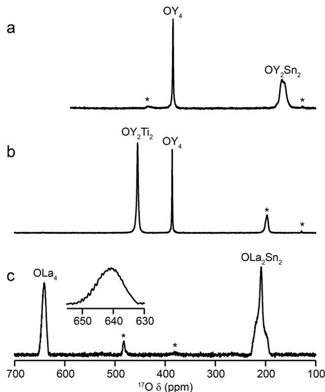
Fig. 2  $^{17}\text{O}$  (14.1 T, 21 kHz) MAS NMR spectra of (a)  $\text{Y}_2\text{Sn}_2\text{O}_7$  (b)  $\text{Y}_2\text{Ti}_2\text{O}_7$  and (c)  $\text{La}_2\text{Sn}_2\text{O}_7$  pyrochlores (enriched at 700 °C for 12 h), with the O coordination environments indicated. Spinning sidebands are shown by \*. In (c), the lineshape of the  $\text{OLa}_4$  resonance is shown expanded.
