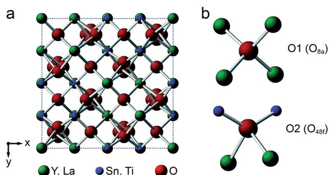
Fig. 1 (a) Structure of a typical  $\text{A}_2\text{B}_2\text{O}_7$  pyrochlore. Red spheres denote O, green spheres, the eight-coordinate A site (occupied by Y or La), and blue spheres, the six-coordinate B site (occupied by Ti or Sn). (b) Expansions showing the coordination environments of the O1 (8a) and O2 (48f) sites.
