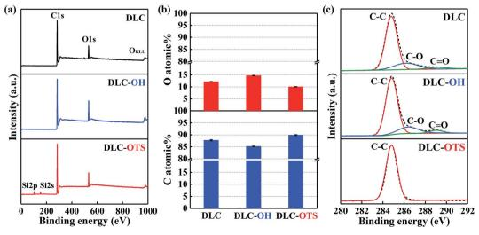
Fig. 2 XPS characterization of DLC films with different modifications: survey spectra (a); C and O atomic% (b); and C1s spectra (c).
