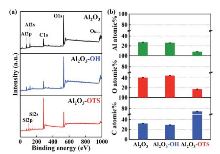
XPS characterization of Al<sub>2</sub>O<sub>3</sub> balls with different modifications: survey spectra (a); C, O, and Al atomic% (b)
