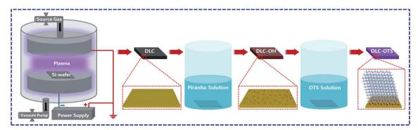
Fig. 1 Schematic view of surface modification of DLC films.
