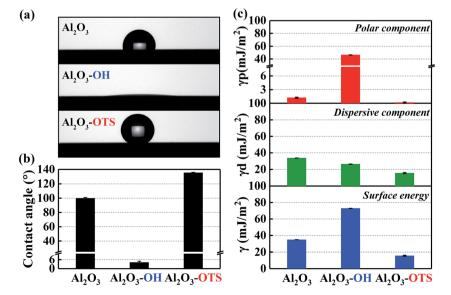
Fig. 5 Digital images of water drop profiles and static water contact angles of Al<sub>2</sub>O<sub>3</sub> balls with different modifications (a) and (b); surface energies and their components of Al<sub>2</sub>O<sub>3</sub> balls with different modifications (c).
