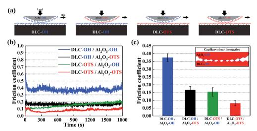
Fig. 6 Schematic view of frictional test with four friction pairs (a); dynamic friction curves (b); mean friction coefficient of four pairs and the inset shows the schematic of capillary force (c).
