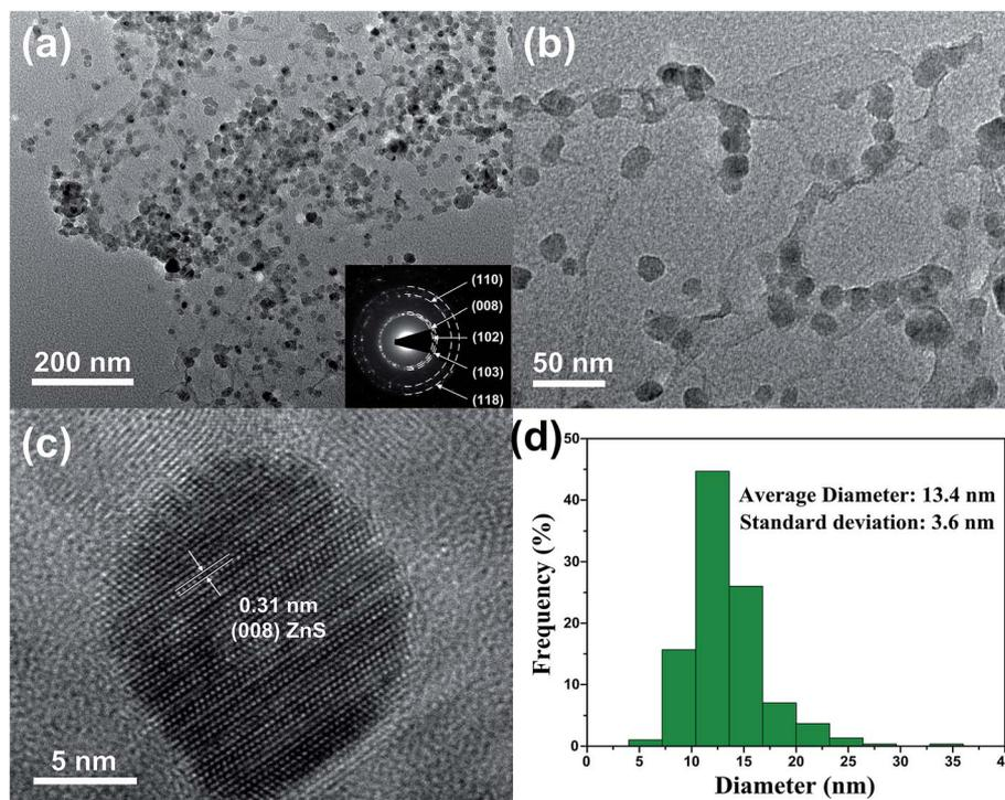
Fig. 5 (a) Low and (b) high magnification TEM images, (c) HRTEM image and (d) particle size distribution of ZSG. Inset of (a) is the corresponding SAED pattern.
