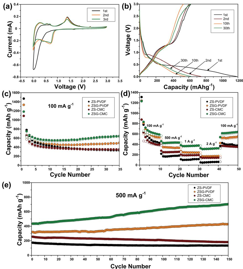
Fig. 6 Electrochemical performance of ZS–PVDF, ZSG–PVDF, ZS–CMC and ZSG–CMC. (a) Cyclic voltammograms of ZSG–CMC in the voltage range of 0.01–3 V at a scan rate of 0.1 mV s<sup>-1</sup>. (b) Galvanostatic charge–discharge profiles of ZSG–CMC at 100 mA g<sup>-1</sup> in 0.01–3 V. (c) Cycling performance and (d) rate capability of ZS–PVDF, ZSG–PVDF, ZS–CMC and ZSG–CMC. (e) Continuous long-term cycling performance of the above four samples after the rate test.
