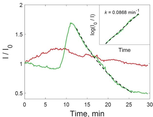
Fig. 5 The intensity of the SERS signal at 1176 cm<sup>-1</sup> registered from a drop of crystal violet solution ( $2 \times 10^{-6}$  M) on a solid substrate (red), or from a drop of the same solution with added hydrogen peroxide (green); the inset shows the linearization of the SERS signal over the range of 12–25 min on a log scale for the drop with added H<sub>2</sub>O<sub>2</sub>.
