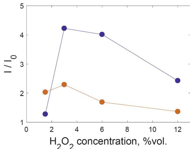
Fig. 4 The intensity of the SERS spectrum at various H<sub>2</sub>O<sub>2</sub> concentrations for crystal violet at 1176 cm<sup>-1</sup> (violet) and rhodamine 6G at 1510 cm<sup>-1</sup> (orange). The lines are a guide for the eye.
