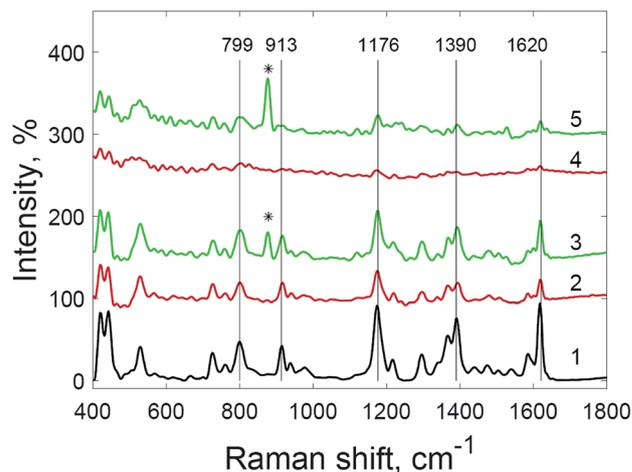
Fig. 8 Raman spectrum of crystal violet (1) and SERS spectra of crystal violet at various concentrations: (2)  $5 \times 10^{-8}$  M; (3)  $5 \times 10^{-8}$  M with hydrogen peroxide; (4)  $5 \times 10^{-9}$  M; and (5)  $5 \times 10^{-9}$  M with hydrogen peroxide (\* = peak from hydrogen peroxide O–O stretching).
