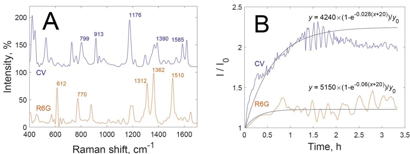
Fig. 1 (A) SERS spectra of  $10^{-6}$  M rhodamine 6G solution (orange) and  $5 \times 10^{-7}$  M crystal violet solution (violet); and (B) experimental (colour) and approximated (black) time dependencies of SERS intensity for rhodamine 6G (orange) and crystal violet (violet) solutions mixed with a dispersion of gold nanoparticles.
