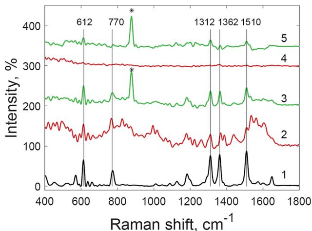
Fig. 9 Raman spectrum of rhodamine 6G (1) and SERS spectra of rhodamine 6G at different concentrations: (2)  $5 \times 10^{-8}$  M; (3)  $5 \times 10^{-8}$  M with hydrogen peroxide; (4)  $5 \times 10^{-9}$  M; and (5)  $5 \times 10^{-9}$  M with hydrogen peroxide (\* = peak from hydrogen peroxide O–O stretching).
