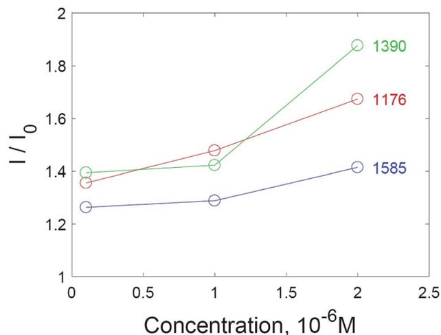
Fig. 7 Normalized intensities of SERS spectra for selected peaks of crystal violet on solid SERS substrates.
