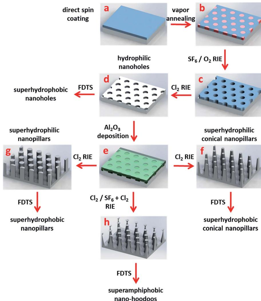
**Fig. 1** (a) Spin coating of PS-PDMS block-copolymer. (b) Solvent annealing. (c) Oxygen plasma ( $O_2$ ) removal of PS blocks and oxidation of PDMS blocks. (d) Shallow nanoholes formed by etching by reactive ion etching in  $Cl_2$ . (e)  $Al_2O_3$  deposition. (f) Formation of high aspect ratio tapered nano-pillars. (g) Formation of straight side-wall nanopillars. (h) Over-hanging nanopillars generated by combined  $Cl_2/SF_6 + Cl_2$  two-step etching.
