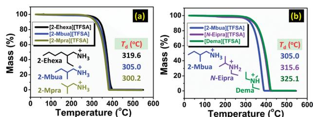
Fig. 1 Thermo-gravimetric curves for PILs with the variation in (a) alkyl chain length, and (b) number of hydrogen bond donors.
