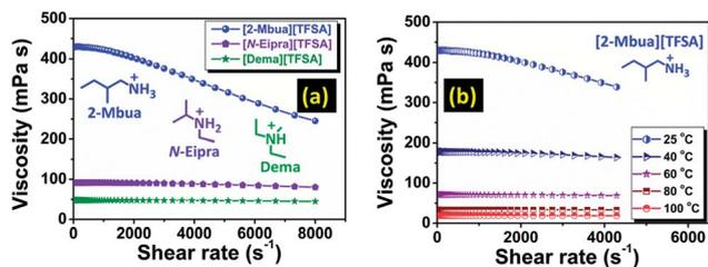
Fig. 3 Change of viscosity as a function of shear rate (a) at 25 °C, (b) under various temperatures. For (b), shear rate was limited to  $4000 \text{ s}^{-1}$  at higher temperatures due to the expelling of the samples at very high shear rate.
