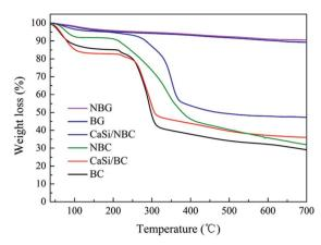
Fig. 7 TGA curves of BC, NBC, CaSi/BC, CaSi/NBC, BG and NBG samples.
