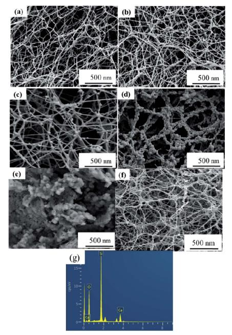
Fig. 3 SEM images of (a) BC, (b) NBC, (c) CaSi/BC, (d) CaSi/NBC, (e) BG and (f) NBG scaffolds, and (g) EDS profile of NBG scaffold as shown in figure (f).
