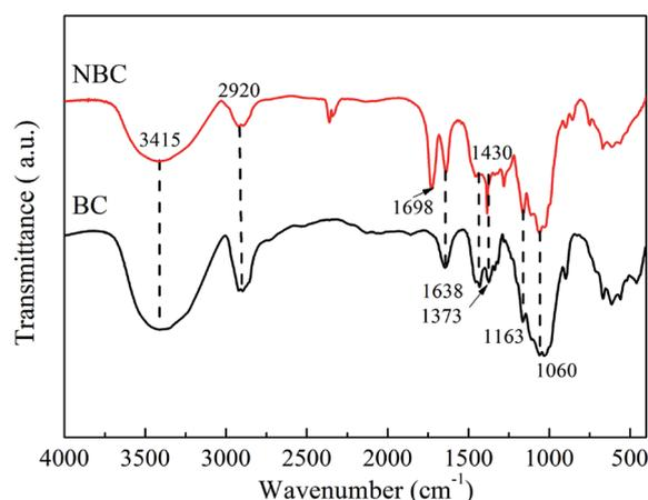
**Fig. 5** FT-IR spectra of BC and NBC samples.
