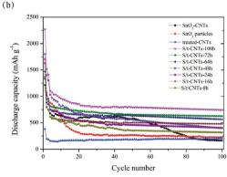
Fig. 4 The selected charge & discharge curves (a) and cycle performance (b) of S/t-CNTs composites, SnO<sub>2</sub>-CNTs and SnO<sub>2</sub> working at current density of  $0.4 \text{ A g}^{-1}$ .
