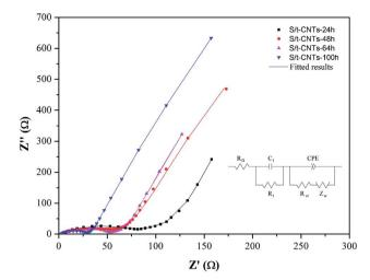
Fig. 6 EIS curves of sample S/t-CNTs-24 h, -48 h, -64 h and -100 h composite.
