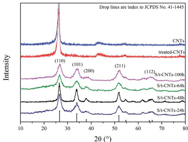
Fig. 1 XRD patterns of S/t-CNTs-24 h, -48 h, -64 h, -100 h, treated-CNTs and CNTs.
