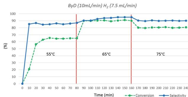
Fig. 6 Influence of temperature on ByD conversion and selectivity to (Z)-BeD under MW irradiation (ByD (10 mL min<sup>-1</sup>) and H<sub>2</sub> (7.5 mL min<sup>-1</sup>)) and 4.5 bar of total pressure.
