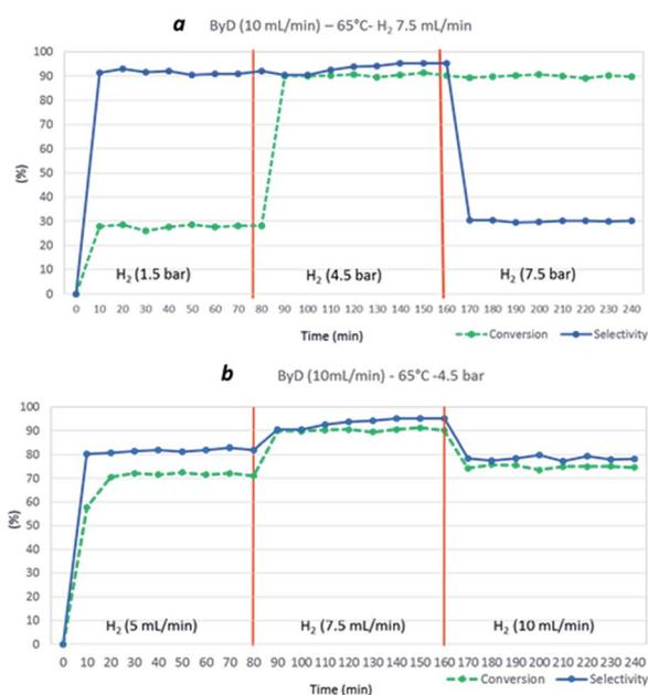
Fig. 5 Influence of H<sub>2</sub> total pressure (at a H<sub>2</sub> flow rate of 7.5 mL min<sup>-1</sup>) (a) and influence of H<sub>2</sub> flow rate (at 4.5 bar) (b) on ByD conversion and selectivity to (Z)-BeD at 65 °C, over a total ByD flow rate of 10 mL min<sup>-1</sup>.
