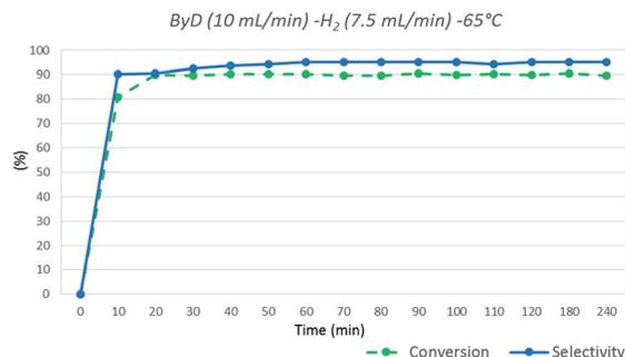
Fig. 3 ByD flow semi-hydrogenation (10 mL min<sup>-1</sup>) at 65 °C and 7.5 (mL min<sup>-1</sup>) H<sub>2</sub> flow and 4.5 bar total pressure.
