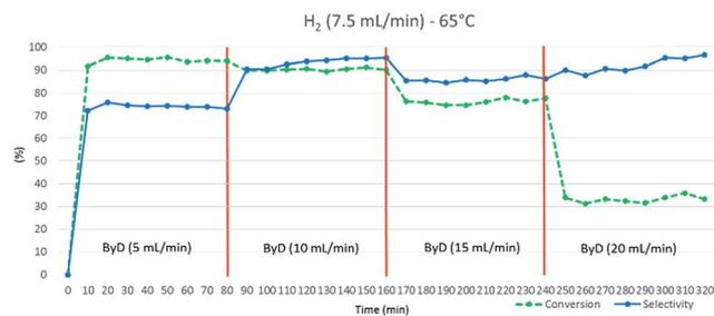
Fig. 4 Influence of ByD flow rate on (Z)-BeD conversion and selectivity at 65 °C, 7.5 (mL min<sup>-1</sup>) H<sub>2</sub> flow and 4.5 bar total pressure.
