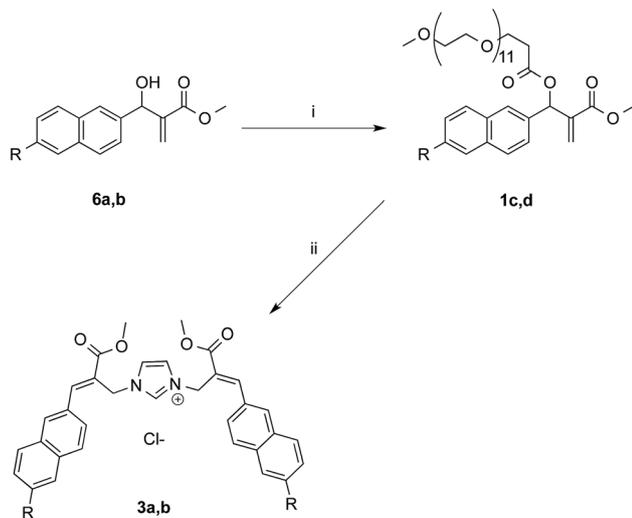
**Scheme 5** Synthesis of water-soluble MBHA derivatives **1c,d** and their reactivity towards imidazole. Reagents: (i)  $\text{CH}_3\text{O}(\text{CH}_2\text{CH}_2\text{O})_{11}\text{CH}_2\text{-CH}_2\text{COCl}$ , TEA,  $\text{CH}_2\text{Cl}_2$ ; (ii) imidazole, PBS. Substituents: R =  $\text{OCH}_2\text{-CCH}$  (**1c**, **3a**, **6a**); CCH (**1d**, **3b**, **6b**).
