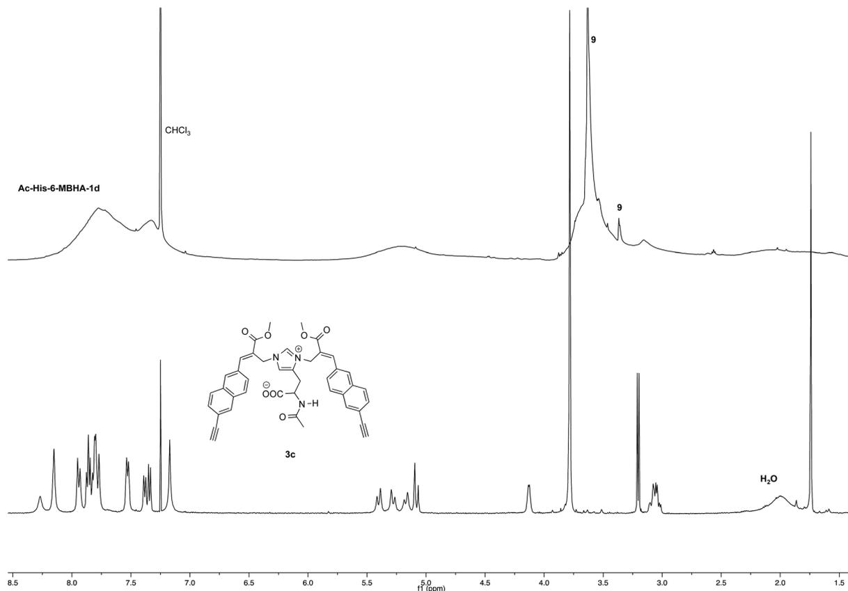
Fig. 5  $^1\text{H}$  NMR spectrum (500 MHz,  $\text{CDCl}_3$ ) of **Ac-His-6-MBHA-1d** obtained by reaction of **Ac-His-6** with a ten-fold excess of **1d** compared with that of biadduct **3c**. The peaks marked by 9 were attributed to compound **9**, which was produced in the concerted addition–elimination process and remained as a counterion of the imidazolium salt moieties.
