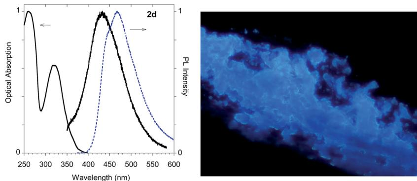
Fig. 12 Optical properties of imidazole derivative **2d**. Left panel: normalized absorption and emission spectra obtained in methanol (black solid line) and emission spectrum of the powder (dashed blue line). Right panel: fluorescence microscopy image (290  $\mu\text{m}$  width) obtained with solid **2d**.
