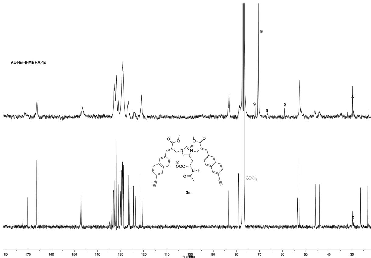
Fig. 6  $^{13}\text{C}$  NMR spectrum (125,  $\text{CDCl}_3$ ) of Ac-His-6-MBHA-1d obtained by reaction of Ac-His-6 with a ten-fold excess of **1d** compared with that of biadduct **3c**. The peaks marked by 9 were attributed to compound **9**, which was produced in the concerted addition–elimination process and remained as a counterion of the imidazolium salt moieties.
