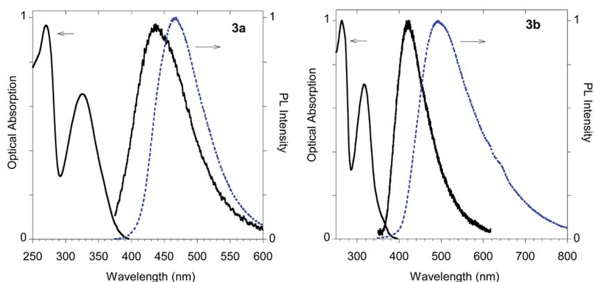
Fig. 13 Optical features of imidazolium salts **3a** and **3b**. Normalized absorption and emission spectra obtained in methanol (black solid line) and emission spectrum of the powder (dashed blue line).
