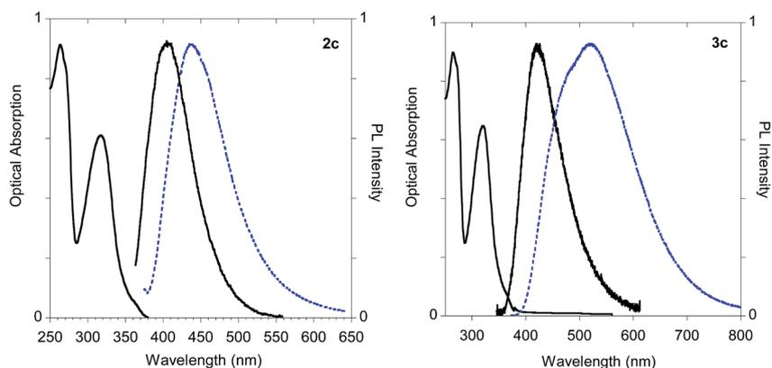
Fig. 14 Optical features of histidine derivatives **2c** and **3c**. Normalized absorption and emission spectra obtained in methanol (black solid line) and emission spectrum of the powder (dashed blue line).
