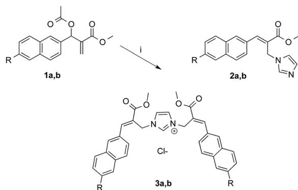
Scheme 3 Reaction of MBHA derivatives **1a,b** with imidazole. Reagents: (i) imidazole, CH<sub>3</sub>CN, PBS. Substituents: R = -OCH<sub>2</sub>CCH (**1a**, **2a**, **3a**); R = -CCH (**1b**, **2b**, **3b**).
