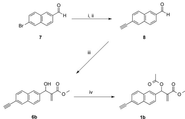
Scheme 2 Synthesis of MBHA derivative **1b**. Reagents: (i) ethynyltrimethylsilane, Pd(PPh<sub>3</sub>)<sub>2</sub>Cl<sub>2</sub>, CuI, TEA, THF; (ii) K<sub>2</sub>CO<sub>3</sub>, MeOH; (iii) DABCO, methyl acrylate, MeOH, THF; (iv) CH<sub>3</sub>COCl, TEA, CH<sub>2</sub>Cl<sub>2</sub>.
