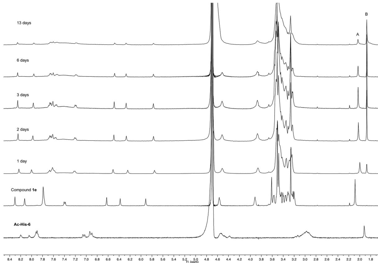
Fig. 7  $^1\text{H}$  NMR spectra (400 MHz,  $\text{PBS-D}_2\text{O}$ ) of the mixtures obtained by reaction of **Ac-His-6** with a ten-fold excess of compound **1e**. The peaks marked with A (attributed to the acetyl moiety of **1e**) and B (attributed to acetate **10** produced by the concerted addition–elimination process) were used to follow the reaction progress.
