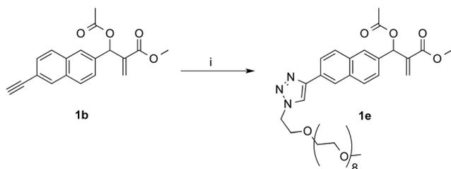
Scheme 7 Synthesis of water-soluble MBHA derivative **1e**. Reagents: (i)  $\text{CH}_3(\text{OCH}_2\text{CH}_2)_9\text{N}_3$ ,  $\text{CuSO}_4$ , sodium ascorbate, *tert*-butanol, PBS.
