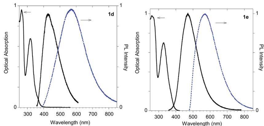
Fig. 15 Optical features of polymeric materials **Ac-His-6-MBHA-1d** and **Ac-His-6-MBHA-1e**. Normalized absorption and emission spectra obtained in methanol (black solid line) and emission spectrum of the powder (dashed blue line).
