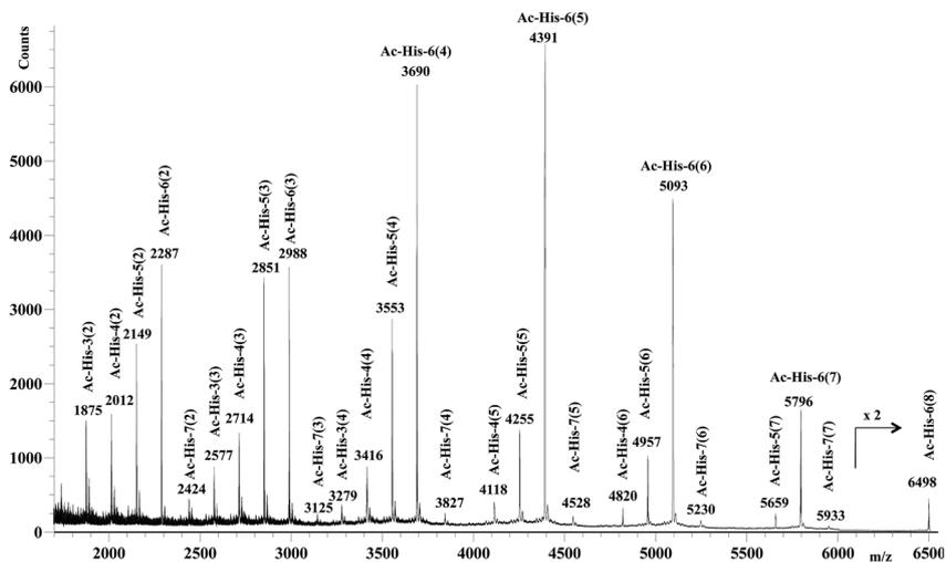
Fig. 8 MALDI-TOF mass spectrum (positive-ion mode) of the polymeric material **Ac-His-6-MBHA-1e** obtained by reaction of **Ac-His-6** with a ten-fold excess of compound **1e**. The polymerization degree of the corresponding **Ac-His** molecule is reported for each monoisotopic mass peak along with the grafting degree (*i.e.* the number of naphthalene substituents for each **Ac-His** molecule) noted in parentheses.
