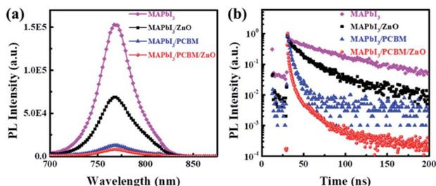
Fig. 3 (a) The steady-state photoluminescence (PL) spectra of MAPbI<sub>3</sub>, MAPbI<sub>3</sub>/ZnO NPs, MAPbI<sub>3</sub>/PC<sub>61</sub>BM and MAPbI<sub>3</sub>/PC<sub>61</sub>BM/ZnO films. The excitation light was set at 610 nm. (b) Time-resolved PL measurements taken at the peak emission wavelength (765 nm) of the various perovskite films. A 5 mW picosecond pulsed diode laser at 638.8 nm excited on glass side of films.
