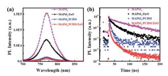
Fig. 3 (a) The steady-state photoluminescence (PL) spectra of MAPbl<sub>3</sub>, MAPbl<sub>3</sub>/ZnO NPs, MAPbl<sub>3</sub>/PC<sub>61</sub>BM and MAPbl<sub>3</sub>/PC<sub>61</sub>BM/ZnO films. The excitation light was set at 610 nm. (b) Time-resolved PL measurements taken at the peak emission wavelength (765 nm) of the various perovskite films. A 5 mW picosecond pulsed diode laser at 638.8 nm excited on glass side of films.
