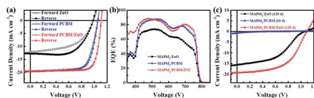
Fig. 2 Current density-voltage (*J*-*V*) curves (a) and external quantum efficiencies (b) of fresh perovskite solar cells with different ETLs. (c) *J*-*V* curves of the devices after storage with a period of 120 days in air with a humidity of 20%. MAPbI<sub>3</sub>/PC<sub>61</sub>BM heterojunction solar cell was only stored 10 days in the same condition.
