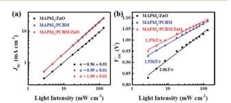
Fig. 4 (a) Measured  $J_{SC}$  of cells with different ETLs plotted against light intensity (symbols) on a logarithmic scale. Fitting a power law (solid lines) to these data yields  $\alpha$ . (b) Measured  $V_{\rm OC}$  of cells with different ETLs plotted against light intensity (symbols), together with linear fits to the data (solid lines).
