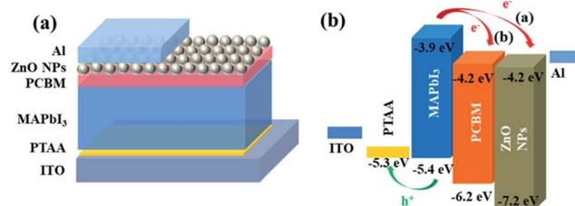
Fig. 1 Schematic illustration of the perovskite solar cell configuration with PC<sub>61</sub>BM/ZnO NPs as ETL (a). (b) The corresponding energy level diagram of the devices.
