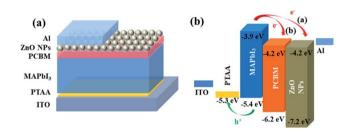
Fig. 1 Schematic illustration of the perovskite solar cell configuration with PC<sub>61</sub>BM/ZnO NPs as ETL (a). (b) The corresponding energy level diagram of the devices.
