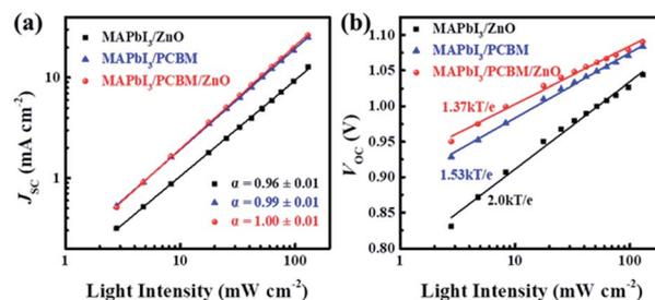
Fig. 4 (a) Measured  $J_{SC}$  of cells with different ETLs plotted against light intensity (symbols) on a logarithmic scale. Fitting a power law (solid lines) to these data yields  $\alpha$ . (b) Measured  $V_{OC}$  of cells with different ETLs plotted against light intensity (symbols), together with linear fits to the data (solid lines).
