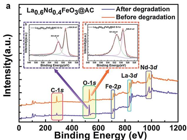
Fig. 6 Survey XPS spectrum and O-1s XPS patterns of the La<sub>0.6</sub>Nd<sub>0.4</sub>FeO<sub>3</sub>@AC composite anode, before and after the electrocatalytic oxidation process.
