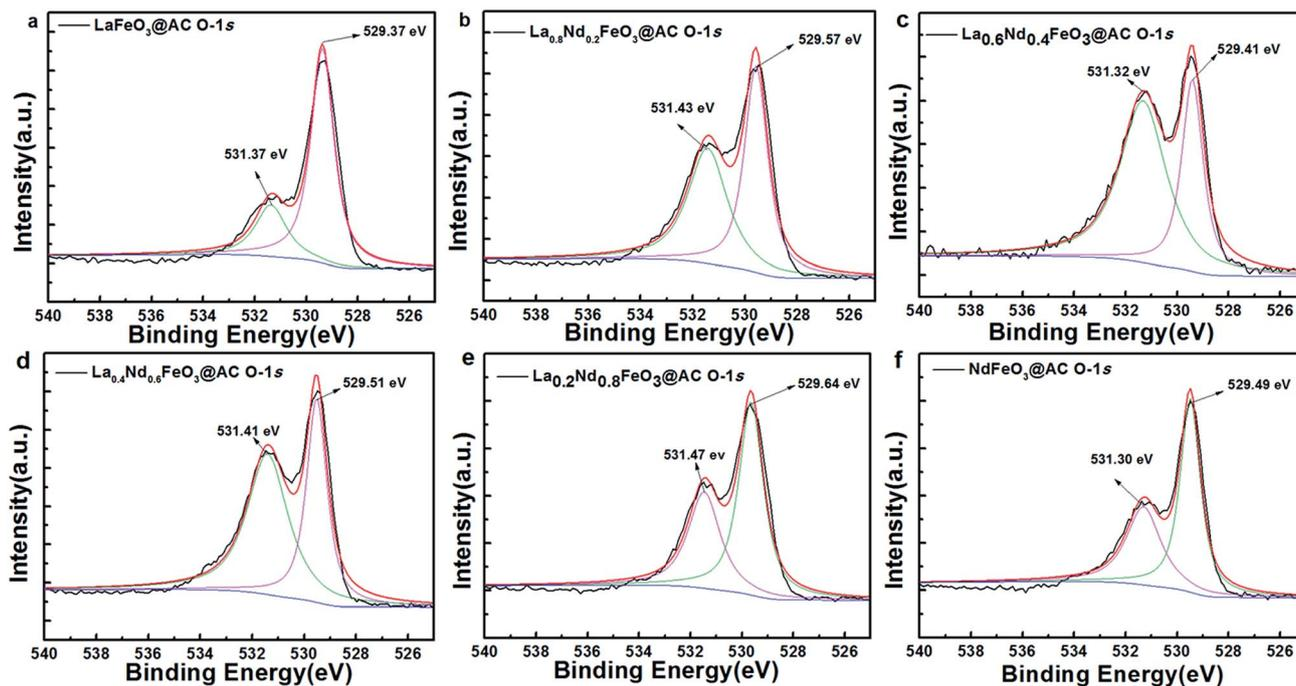
Fig. 5 O-1s XPS patterns of the perovskite catalysts: (a) LaFeO<sub>3</sub>@AC; (b) La<sub>0.8</sub>Nd<sub>0.2</sub>FeO<sub>3</sub>@AC; (c) La<sub>0.6</sub>Nd<sub>0.4</sub>FeO<sub>3</sub>@AC; (d) La<sub>0.4</sub>Nd<sub>0.6</sub>FeO<sub>3</sub>@AC; (e) La<sub>0.2</sub>Nd<sub>0.8</sub>FeO<sub>3</sub>@AC; (f) NdFeO<sub>3</sub>@AC.
