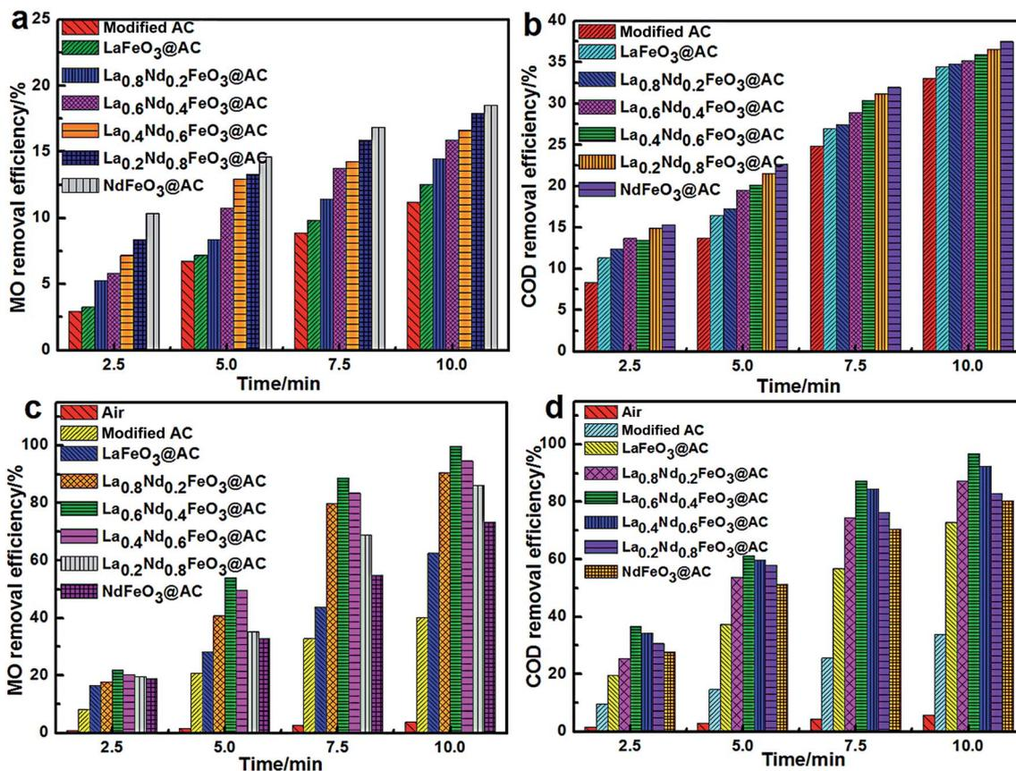
Fig. 7 (a) The MO removal efficiency in MO wastewater of different composite anodes (physical adsorption); (b) the COD removal efficiency in MO wastewater of different composite anodes (physical adsorption); (c) the MO removal efficiency in MO wastewater of different composite anodes and air during the electrocatalytic process; (d) the COD removal efficiency in MO wastewater of different composite anodes and air during the electrocatalytic process.
