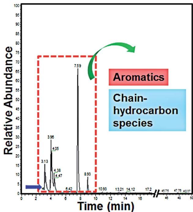
Fig. 11 GC-MS spectrum of MO wastewater after degradation by a La<sub>0.6</sub>Nd<sub>0.4</sub>FeO<sub>3</sub>@AC composite anode for 10 min.
