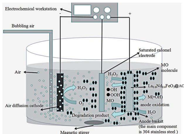
Fig. 12 Mechanism of MO degradation by a La<sub>0.6</sub>Nd<sub>0.4</sub>FeO<sub>3</sub>@AC composite anode.
