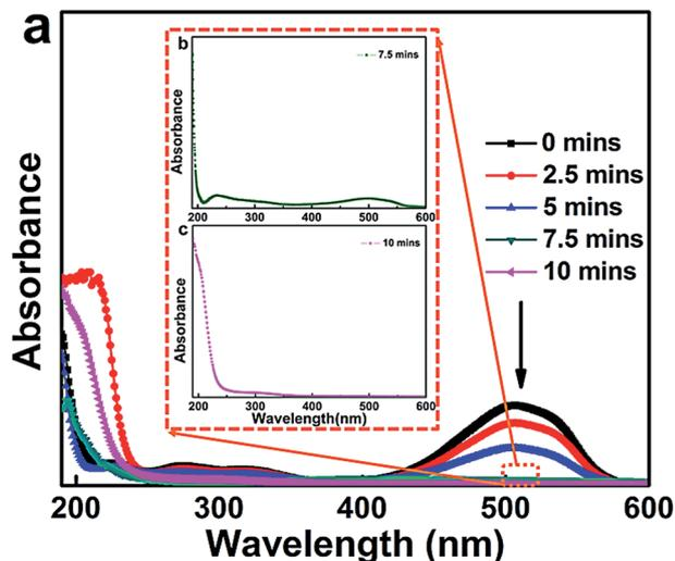
Fig. 10 UV-vis spectral changes of the 500 mg L<sup>-1</sup> MO solution during the degradation process as a function of reaction time in the presence of 7 g L<sup>-1</sup> Na<sub>2</sub>SO<sub>4</sub>, *I* = 400 mA dm<sup>-2</sup> and pH = 2.0.
