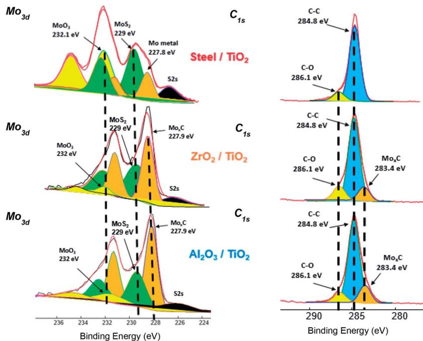
Fig. 15 Comparison of high resolution XPS Mo3d and C1s spectra for TiO<sub>2</sub> APS flats (right) sliding against steel, ZrO<sub>2</sub> and Al<sub>2</sub>O<sub>3</sub> balls respectively (from top to bottom) at maximum contact pressure of 0.7 GPa lubricated with base oil + 0.3% MoDTC at a constant temperature of 100 °C.
