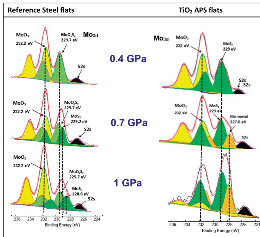
Fig. 11 Comparison of high resolution XPS Mo3d spectra for reference steel (left) and TiO<sub>2</sub> APS flats (right) at different pressures of 0.4 GPa, 0.7 GPa and 1 GPa lubricated with base oil + 0.3% MoDTC at a constant temperature of 100 °C.
