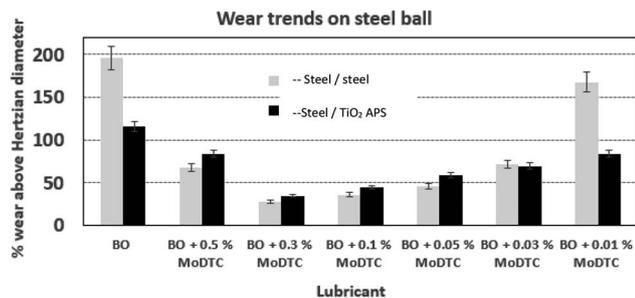
Fig. 4 Comparison of wear trends on the steel ball tested against reference steel and TiO<sub>2</sub> APS flats lubricated with various concentrations of MoDTC in base oil (tribotest at 100 °C, at 0.05 m s<sup>-1</sup>, with maximum contact pressure of 700 MPa).
