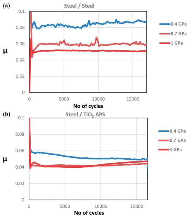
Fig. 9 Comparison of friction behavior at different pressures for (a) steel/steel (b) steel/TiO<sub>2</sub> APS.
