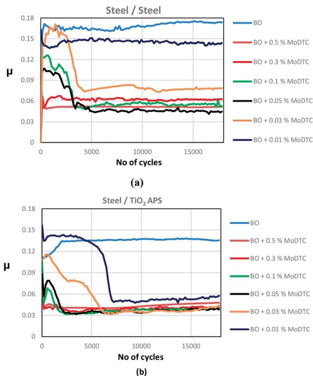
Fig. 3 Friction curves obtained after tests at 100 °C, at 0.05 m s<sup>-1</sup>, with maximum contact pressure of 700 MPa and at various concentrations of MoDTC in base oil for (a) steel/reference steel (b) steel/TiO<sub>2</sub> APS.
