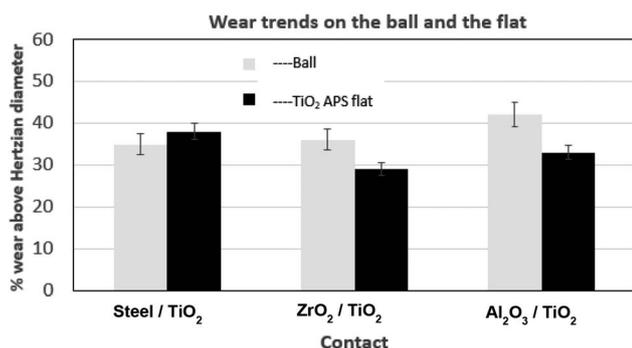
Fig. 14 Comparison of wear trends on the various balls tested against TiO<sub>2</sub> APS flats lubricated with base oil + 0.3% MoDTC at a pressure of 0.7 GPa and temperature of 100 °C.
