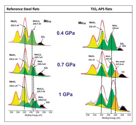
Fig. 11 Comparison of high resolution XPS Mo3d spectra for reference steel (left) and  $TiO_2$  APS flats (right) at different pressures of 0.4 GPa, 0.7 GPa and 1 GPa lubricated with base oil + 0.3% MoDTC at a constant temperature of 100 °C.
