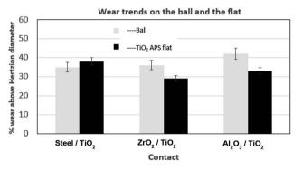
Fig. 14 Comparison of wear trends on the various balls tested against  $TiO_2$  APS flats lubricated with base oil + 0.3% MoDTC at a pressure of 0.7 GPa and temperature of 100 °C.
