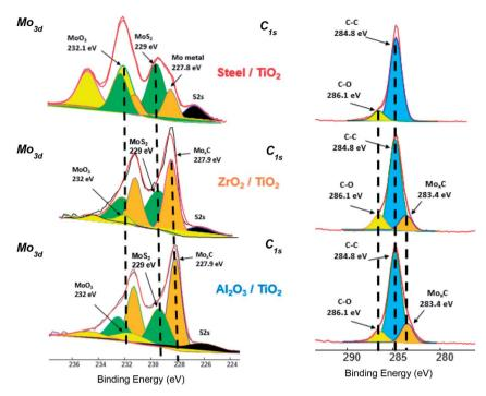
Fig. 15 Comparison of high resolution XPS Mo3d and C1s spectra for  $TiO_2$  APS flats (right) sliding against steel,  $ZrO_2$  and  $Al_2O_3$  balls respectively (from top to bottom) at maximum contact pressure of 0.7 GPa lubricated with base oil + 0.3% MoDTC at a constant temperature of 100 °C.
