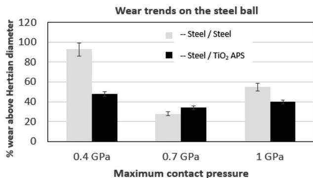
Fig. 10 Comparison of wear trends on the steel ball tested against reference steel and TiO<sub>2</sub> APS flats lubricated with base oil + 0.3% MoDTC at different contact pressures (0.4 GPa, 0.7 GPa and 1 GPa).
