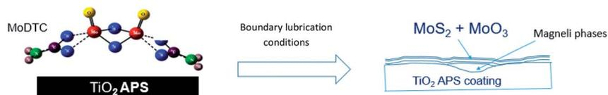
Fig. 2 Schematic highlighting the compounds obtained after friction test under boundary lubrication conditions in presence of MoDTC and TiO<sub>2</sub> APS coating (0.7 GPa Hertzian maximum pressure, 100 °C, 0.5 wt% MoDTC in base oil).
