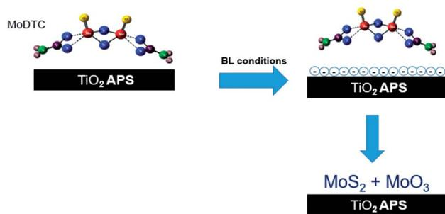
Fig. 16 Schematic of the decomposition mechanism of MoDTC in steel/TiO<sub>2</sub> APS contacts.
