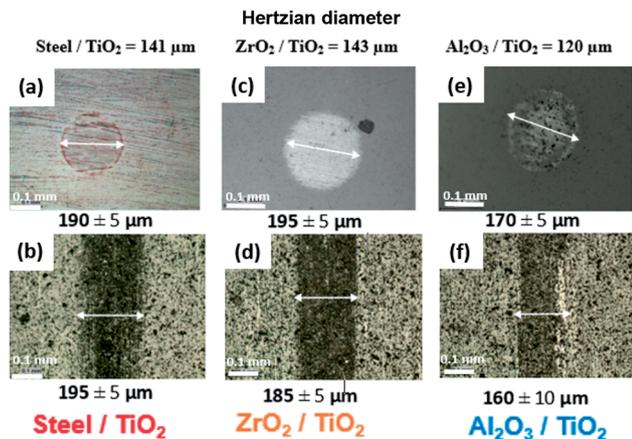
Fig. 13 Optical images of the wear scars on (a) steel ball vs. reference steel flat, (b) steel flat, (c) steel ball vs. TiO<sub>2</sub> flat, (d) TiO<sub>2</sub> flat, (e) steel ball vs. steel APS, (f) steel APS flat when lubricated with base oil + MoDTC.
