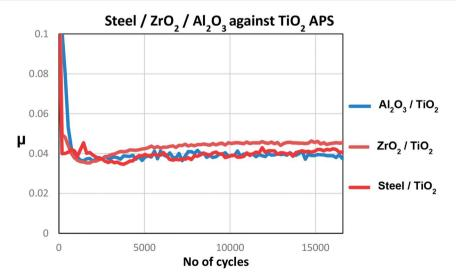
Fig. 12 Comparison of friction behaviour for steel/ $TiO_2$  APS,  $ZrO_2/TiO_2$  APS and  $Al_2O_3/TiO_2$  APS at a maximum Hertzian contact pressure of 0.7 GPa lubricated with base oil + 0.3% MoDTC and a constant temperature of 100 °C.
