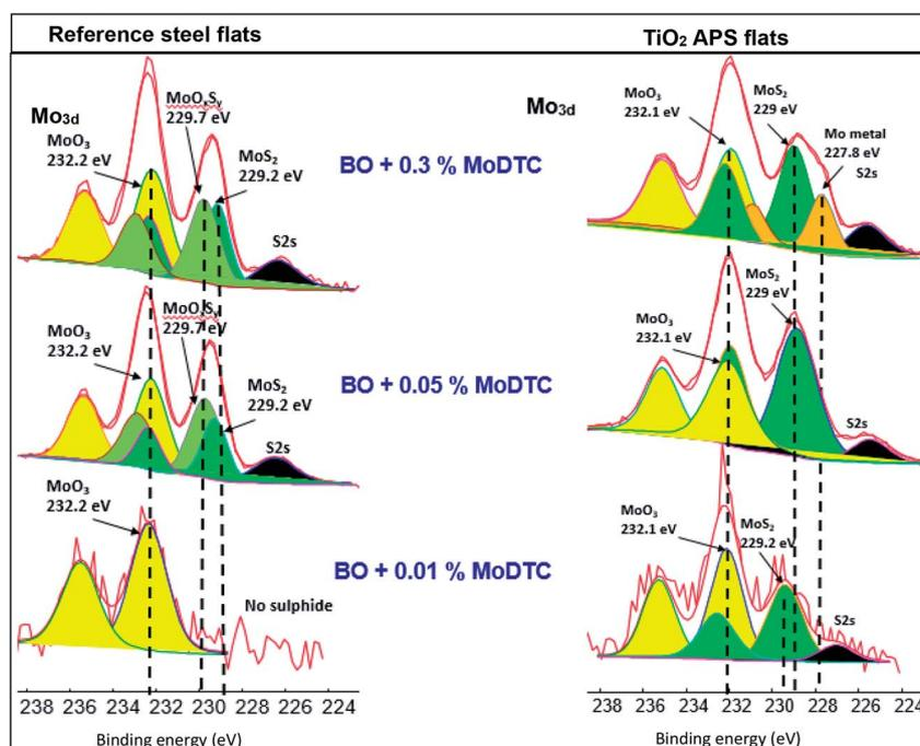
Fig. 5 Comparison of high resolution Mo3d XPS spectra for reference steel (left) and TiO<sub>2</sub> APS flats (right) lubricated with (from the top) base oil + 0.3wt%, base oil + 0.05 wt% and base oil + 0.01 wt% MoDTC (tribotest at 100 °C, at 0.05 m s<sup>-1</sup>, with maximum contact pressure of 700 MPa).
