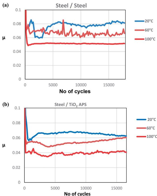
Fig. 6 Comparison of friction behaviour for (a) steel/steel (b) steel/TiO<sub>2</sub> APS at different temperatures (tribotests at 0.05 m s<sup>-1</sup>, with maximum contact pressure of 700 MPa, with 0.3 wt% of MoDTC in base oil).
