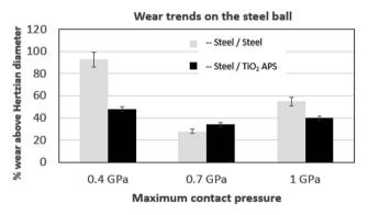
Fig. 10 Comparison of wear trends on the steel ball tested against reference steel and  $TiO_2$  APS flats lubricated with base oil + 0.3% MoDTC at different contact pressures (0.4 GPa, 0.7 GPa and 1 GPa).
