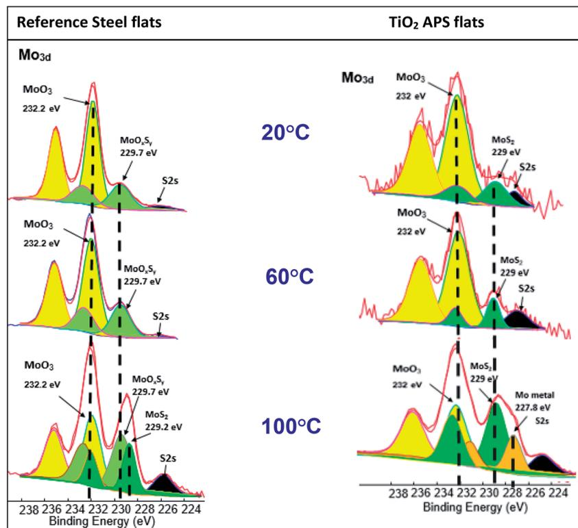
Fig. 8 Comparison of high resolution XPS Mo3d spectra for reference steel (left) and TiO<sub>2</sub> APS flats (right) at different temperatures of 20 °C, 60 °C and 100 °C lubricated with base oil + 0.3% MoDTC at a maximum Hertzian contact pressure of 700 MPa and at a speed of 0.05 m s<sup>-1</sup>.
