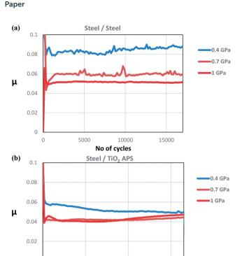
Fig. 9 Comparison of friction behavior at different pressures for (a) steel/steel (b) steel/TiO<sub>2</sub> APS.
