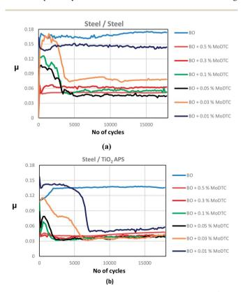
Fig. 3 Friction curves obtained after tests at  $100 \,^{\circ}$ C, at  $0.05 \, \text{m s}^{-1}$ , with maximum contact pressure of 700 MPa and at various concentrations of MoDTC in base oil for (a) steel/reference steel (b) steel/TiO<sub>2</sub> APS.
