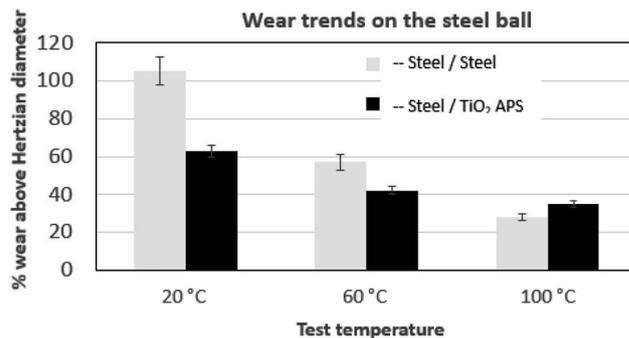
Fig. 7 Comparison of wear trends on the steel ball tested against reference steel and TiO<sub>2</sub> APS flats lubricated with base oil + 0.3% MoDTC at different temperatures (20 °C, 60 °C and 100 °C).
