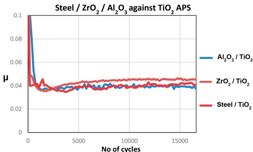
Fig. 12 Comparison of friction behaviour for steel/TiO<sub>2</sub> APS, ZrO<sub>2</sub>/TiO<sub>2</sub> APS and Al<sub>2</sub>O<sub>3</sub>/TiO<sub>2</sub> APS at a maximum Hertzian contact pressure of 0.7 GPa lubricated with base oil + 0.3% MoDTC and a constant temperature of 100 °C.
