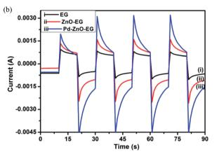
Fig. 3 (a) Cyclic voltammograms of (i) EG, (ii) ZnO-EG and (iii) Pd-ZnO-EG electrodes in 5 mM  $[Fe(CN)_6]^{-3/-4}$ , 0.1 M KCl solution, at 50 mV s<sup>-1</sup> scan rate (b) photocurrent responses of (i) EG, (ii) ZnO-EG and (iii) Pd-ZnO-EG electrodes in the dark and under light.
