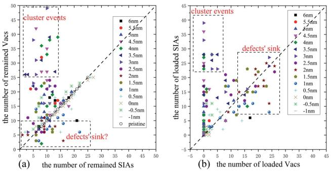
Fig. 3 The number of Vacs and SIAs (a) remained in the crystal or (b) loaded along the ED in pristine bcc Fe and in bcc Fe with an ED after 5 keV collision cascades at 300 K. Each point corresponds to a simulation run. (a) The white circles along the dash line represent 50 simulations in pristine samples.
