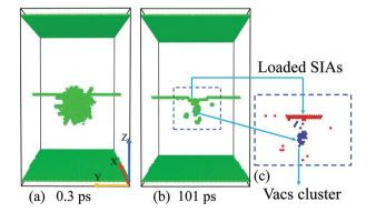
Fig. 5 Temporal evolution of the situation B: formation of a large vacancy cluster. (a) When the peak cascade is just hanging on the dislocation line, enormous SIAs are loaded along the ED, which facilitates the formation of a large vacancy cluster (containing 34 Vacs) in (c), accompanied with the climbing down of the dislocation line (b).
