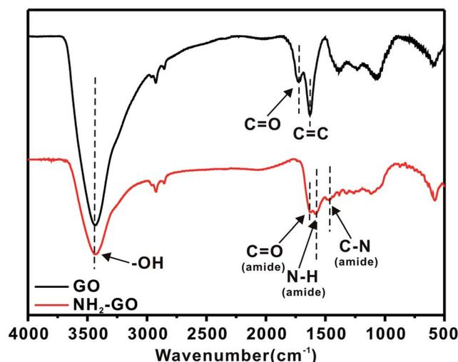
Fig. 3 FT-IR spectra of GO and  $\text{NH}_2\text{-GO}$ .
