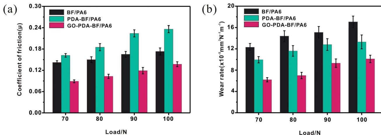
Fig. 9 Friction coefficient (a) and wear rate (b) of BF/PA6, PDA-BF/PA6, and GO-PDA-BF/PA6 composites as a function of applied load ( $0.167 \text{ m s}^{-1}$ , 30 min).
