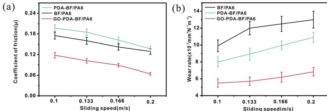
Fig. 10 Friction coefficient (a) and wear rate (b) of BF/PA6, PDA-BF/PA6, and GO-PDA-BF/PA6 composites as a function of sliding speed (70 N, 30 min).
