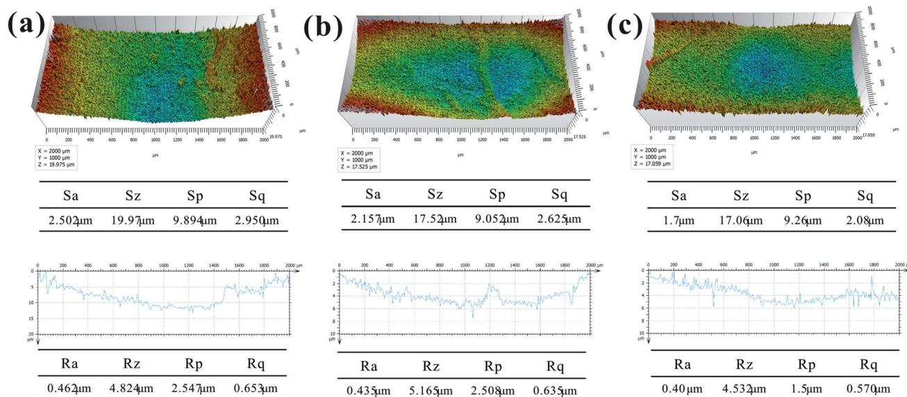
Fig. 13 3D topographies of worn surface: (a) BF/PA6, (b) PDA-BF/PA6 and (c) GO-PDA-BF/PA6.
