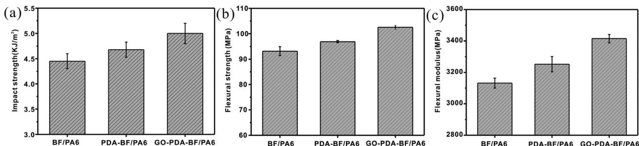
Fig. 6 Impact strength (a), flexural strength (b) and flexural modulus (c) of BF/PA6, PDA-BF/PA6 and GO-PDA-BF/PA6 composites.
