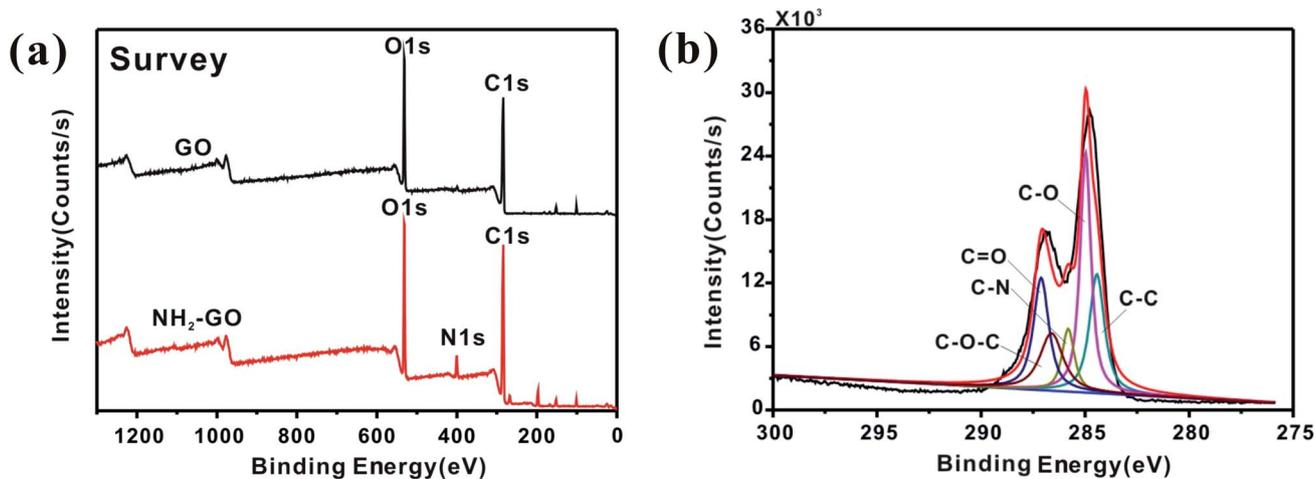
Fig. 4 XPS wide-scan (a) and C 1s core-level spectra (b) of NH<sub>2</sub>-GO.
