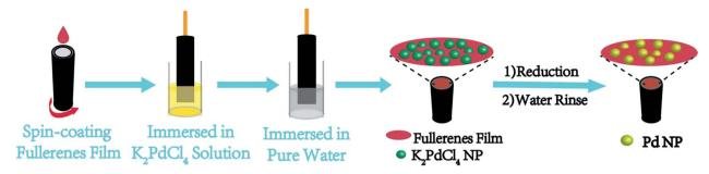
Fig. 6 Procedure for *in situ* fabrication of an immobilized Pd nanoparticle electrocatalyst on a working electrode using PCBANI and PCBDANI as conductive supports.
