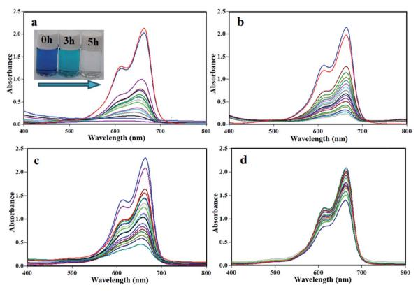
Fig. 10 UV-Vis spectral changes of MB aqueous solutions over different catalysts: (a) m-APO/ $C_{60}$ (5), (b) m-APO/ $C_{60}$ (10), (c) m-APO/ $C_{60}$ (20) and (d) pure APO under visible light. The inset photo in (a) shows the color change of the MB solution during photodegradation. Experimental conditions: [MB] = 25 mg L<sup>-1</sup>, [catalyst] = 0.05 g and [H<sub>2</sub>O<sub>2</sub>] = 30 wt%, 0.5 mL under visible light irradiation for 5 h.
