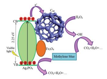
Fig. 12 A proposed mechanism for the photocatalytic degradation of MB over the m-APO/C<sub>60</sub> nanocomposite.
