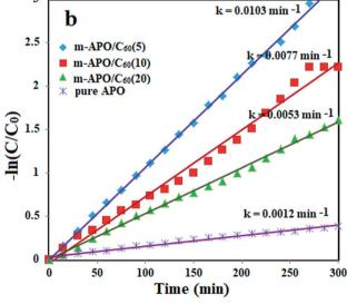
Fig. 11 (a) Concentration changes  $(C/C_0)$  and (b) plot of  $-\ln(C/C_0)$ versus irradiation time of MB dye over APO/C<sub>60</sub>(5), m-APO/C<sub>60</sub>(10), m-APO/C<sub>60</sub>(20) and pure APO photocatalysts. Experimental conditions: [MB] = 25 mg  $L^{-1}$ , [catalyst] = 0.05 g and [H<sub>2</sub>O<sub>2</sub>] = 30 wt%, 0.5 mL under visible light irradiation for 5 h.
