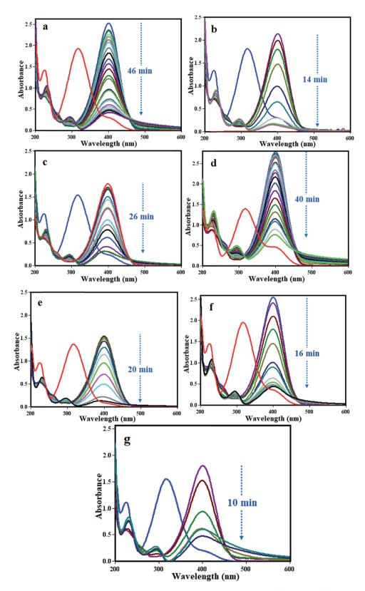
Fig. 15 UV-Vis spectral changes during the reduction of 4-NP with NaBH<sub>4</sub> over different catalysts: (a) pure APO, (b) m-APO- $C_{60}(5)$ , (c) m-APO- $C_{60}(10)$ , (d) m-APO- $C_{60}(20)$ , (e) m-APO- $C_{60}(5)$  and (g) APO- $C_{60}(10)$ . Experimental conditions: [4-NP] = 0.2 mM, [catalyst] = 2.5 mg and [NaBH<sub>4</sub>] = 20 mM, 0.5 ml at 25 °C.
