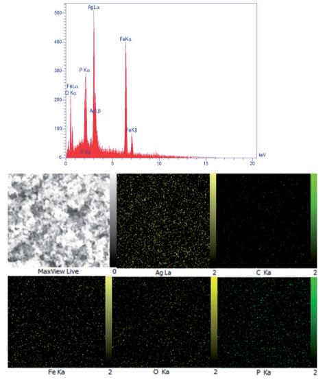
Fig. 5 EDX spectrum and elemental mapping of the m-APO/C<sub>60</sub>(5) nanocomposite.
