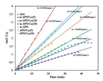
Fig. 14 The plot of  $-\ln(C/C_0)$  versus reduction time for the reduction of 4-NP in the presence of the different catalysts. Experimental conditions: [4-NP] = 0.2 mM, [catalyst] = 2.5 mg and [NaBH<sub>4</sub>] = 20 mM, 0.5 ml at 25 °C.
