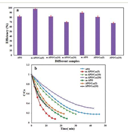
Fig. 13 (a) Comparison of the reduction efficiencies of 4-NP with NaBH<sub>4</sub> over different catalysts, and (b) concentration changes ( $C/C_0$ ) of 4-NP as a function of time. Experimental conditions: [4-NP] = 0.2 mM, [catalyst] = 2.5 mg and [NaBH<sub>4</sub>] = 20 mM, 0.5 ml at 25 °C.
