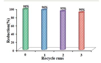
Fig. 17 Recycling experiments for the m-APO- $C_{60}(5)$  nanocomposite in the catalytic reduction of 4-NP.
