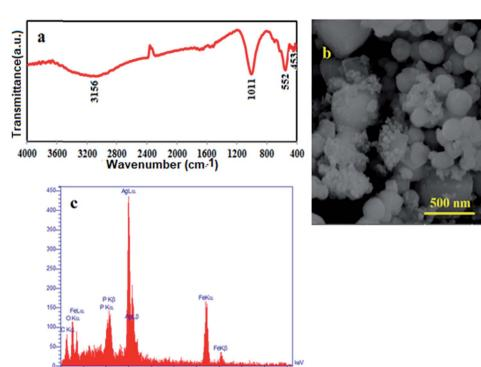
Fig. 18 (a) FT-IR spectrum, (b) SEM image and (c) EDX analysis of the recycled m-APO/C<sub>60</sub>(5) catalyst.
