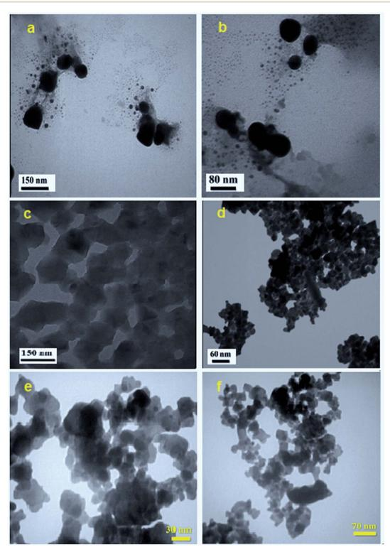
Fig. 6 TEM images of (a and b) pure APO, (c)  $C_{60}$ , (d)  $Fe_3O_4$  and (e and f) m-APO/ $C_{60}$ (5).
