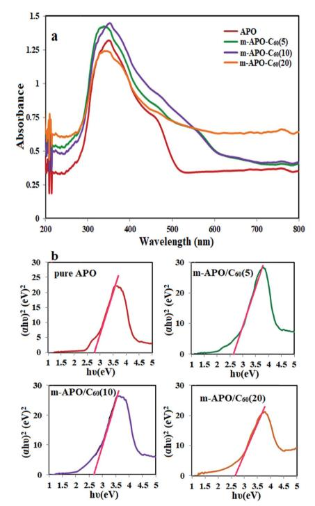
Fig. 9 (a) The UV-Vis diffuse reflectance spectra and (b)  $(\alpha h \nu)^2 - (h \nu)$  curves for pure APO and the m-APO/C<sub>60</sub>(5), m-APO/C<sub>60</sub>(10) and m-APO/C<sub>60</sub>(20) nanocomposites.
