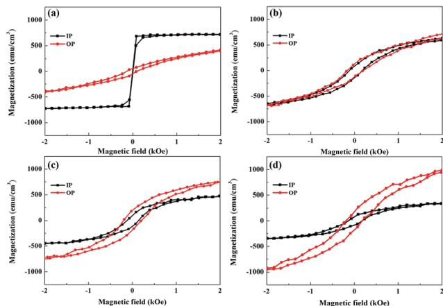
Fig. 5 Room temperature magnetic properties.  $M-H$  curves with  $\text{Bi}_2\text{Se}_3$  thickness-dependence measured at 300 K, along the in-plane (IP) and out-of-plane (OP) directions: (a) pure Py, (b)  $\text{Py}/\text{Bi}_2\text{Se}_3$ -5 nm, (c)  $\text{Py}/\text{Bi}_2\text{Se}_3$ -20 nm and (d)  $\text{Py}/\text{Bi}_2\text{Se}_3$ -40 nm. All the  $M-H$  curves were normalized to the sample area to ensure a reasonable quantitative comparison.
