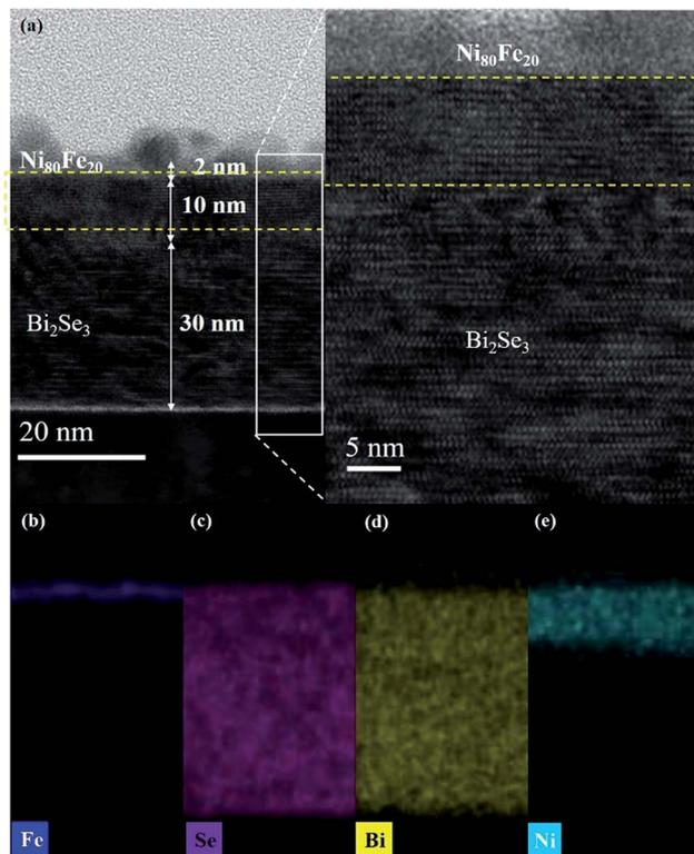
Fig. 3 TEM characterization and EDX chemical mapping of the Py/ $\text{Bi}_2\text{Se}_3$  heterostructure. (a) Cross-sectional TEM image of the heterostructure. EDX mapping of (b) Fe, (c) Se, (d) Bi and (e) Ni. The inset in (a) is an HRTEM image of the selected region of the heterostructure, in which the dashed lines identify the intermediate phases with crystallinity and lattice spacing different from those of amorphous Py (top) and epitaxial  $\text{Bi}_2\text{Se}_3$  (bottom).
