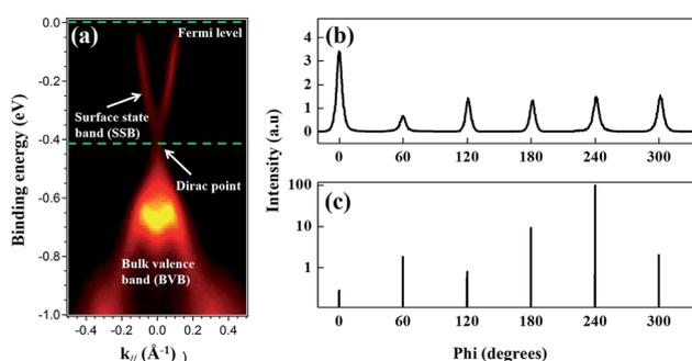
Fig. 1 X-ray characterization of the electronic and structural properties. (a) ARPES spectra of Bi<sub>2</sub>Se<sub>3</sub> film taken along the  $\Gamma$ -K direction, identifying details of the band structure (Fermi-level, surface state band, Dirac point and bulk valence band). X-ray azimuthal scans of the: (b) Bi<sub>2</sub>Se<sub>3</sub> film and (c) sapphire substrate.
