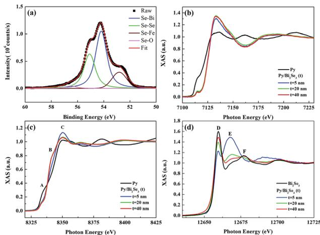
Fig. 4 SR-PES and XANES of the Py/Bi<sub>2</sub>Se<sub>3</sub> heterostructure. (a) SR-PES Se 3d spectrum of Py/Bi<sub>2</sub>Se<sub>3</sub>-40 nm heterostructure after Ar ion etching for 8 min at 2 keV, showing curve-fitting for Se–Bi, Se–Se, Se–Fe, Se–O bonding; (b) Fe K-edge, (c) Ni K-edge, and (d) Se K-edge XANES spectra with Bi<sub>2</sub>Se<sub>3</sub> thickness-dependence.
