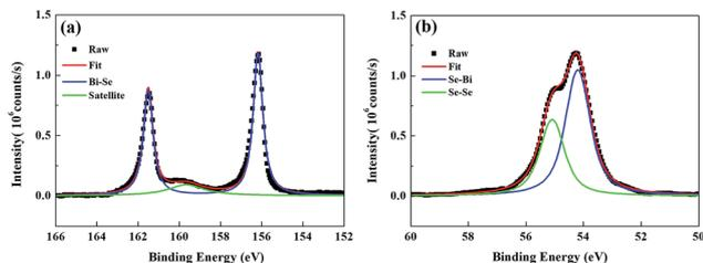
Fig. 2 SR-PES spectra of the  $\text{Bi}_2\text{Se}_3$  film. (a) Bi-4f and (b) Se-3d doublet peaks with curve fittings. The incident energy was fixed at 380 and 250 eV for Bi-4f and Se-3d, respectively.
