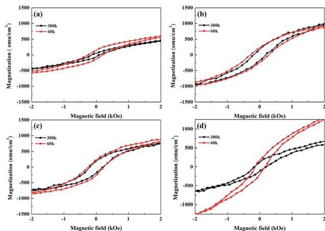
Fig. 6 Temperature-dependent magnetic properties. Out-of-plane  $M-H$  curves with  $\text{Bi}_2\text{Se}_3$  thickness-dependence measured at 60 and 300 K, for: (a) pure Py, (b)  $\text{Py}/\text{Bi}_2\text{Se}_3$ -5 nm, (c)  $\text{Py}/\text{Bi}_2\text{Se}_3$ -20 nm and (d)  $\text{Py}/\text{Bi}_2\text{Se}_3$ -40 nm. All the  $M-H$  curves were normalized to the sample area to ensure a reasonable quantitative comparison.
