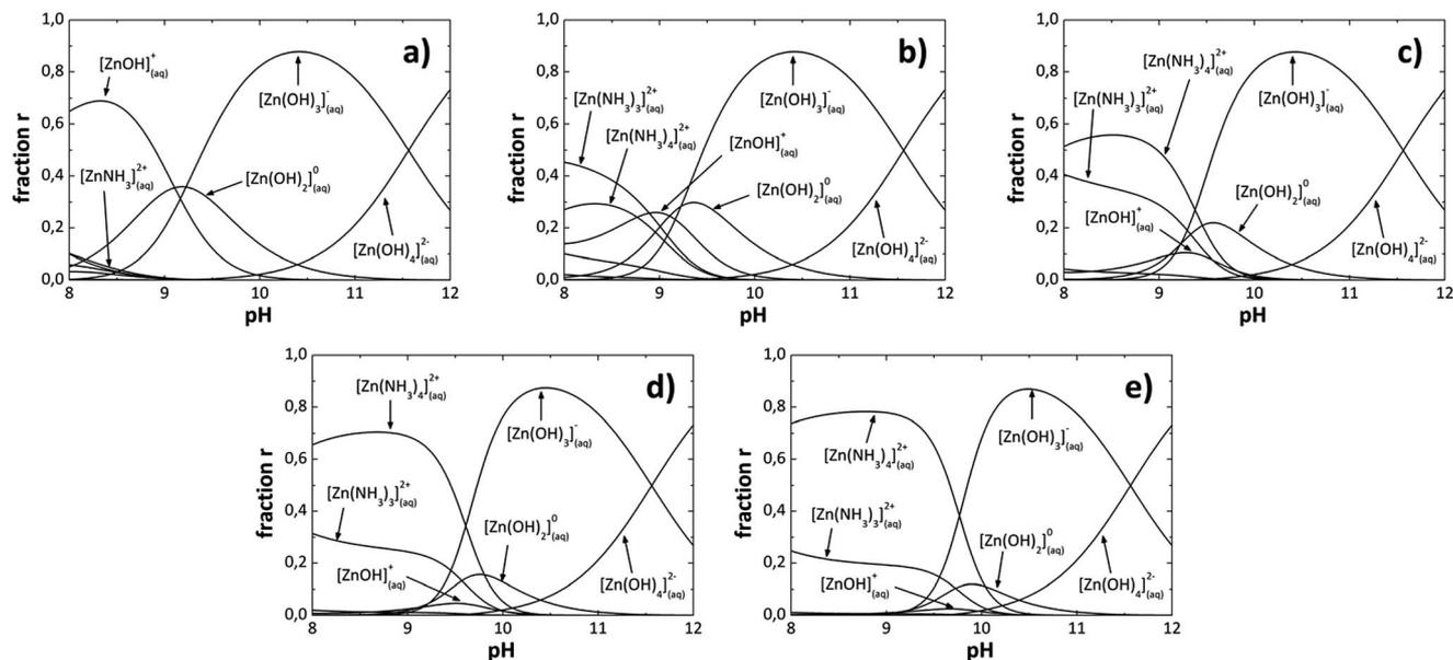
Fig. 1 Species diagrams at 80 °C for: (a)  $1.77 \times 10^{-5}$ , (b)  $7.58 \times 10^{-5}$ , (c)  $2.45 \times 10^{-4}$ , (d)  $8.70 \times 10^{-4}$  and (e)  $1.38 \times 10^{-3}$ ,  $\text{OH}^-$  ions concentration.
