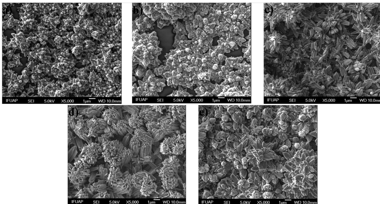
Fig. 3 SEM images of ZnO structures grown by MWCBD technique using the  $[\text{OH}^-]$ ; (a)  $1.77 \times 10^{-5}$ , (b)  $7.58 \times 10^{-5}$ , (c)  $2.45 \times 10^{-4}$ , (d)  $8.70 \times 10^{-4}$  and (e)  $1.38 \times 10^{-3}$ .
