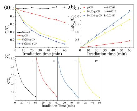
Fig. 7 Photocatalytic performances (a) and corresponding first-order reaction kinetics (b) in the degradation of RhB under visible light irradiation for the pure  $g-C_3N_4$ , the  $Fe(\shortparallel)-g-C_3N_4$  and  $Fe(\shortparallel)/S-g-C_3N_4$ . Stability test of the  $Fe(\shortparallel)/S-g-C_3N_4$  (c).
