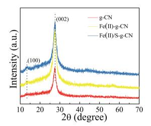
Fig. 2  $\,$  XRD patterns of the g-C  $_3N_4,$  Fe(II) doped and Fe(II)/S codoped of g-C  $_3N_4$  catalysts.
