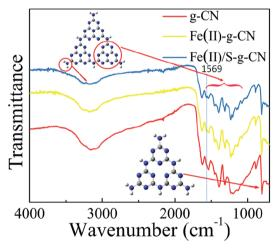
Fig. 3 FT-IR spectra of the pure, Fe(II) doped and Fe(II)/S codoped of  $g\text{-}C_3N_4.$
