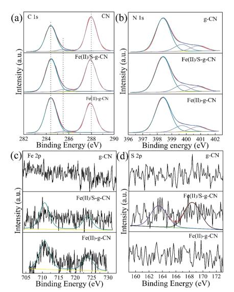
Fig. 4 XPS high resolution spectra for C 1s (a) and N 1s (b), Fe 2p (c) and S 2p (d) of the pure  $g-C_3N_4$  nanosheets (g-CN) and Fe(II) doped  $g-C_3N_4$  (Fe(II)-g-CN) and Fe(II) + S codoped  $g-C_3N_4$  (Fe(II)/S-g-CN).
