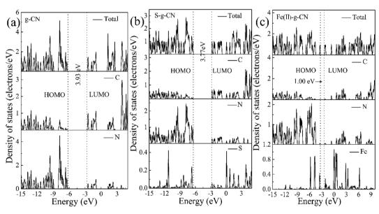
Fig. 10 Calculated total and partial DOS plots of C, N, S and Fe(n) elements for the pristine (a), S doped (b) and (c) Fe(n) doped  $g-C_3N_4$  monolayer.
