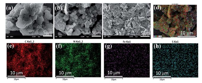
Fig. 1 SEM images of (a) the pure, (b) Fe( $_{\parallel}$ )/S and (c) Fe( $_{\parallel}$ ) doped g-C<sub>3</sub>N<sub>4</sub> photocatalysts. Elemental EDX overlapped images of C, N, Fe and S (d) and mappings for C (e), N (f), Fe (g) and S (h) for the Fe( $_{\parallel}$ )/S codoped g-C<sub>3</sub>N<sub>4</sub>.
