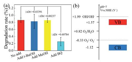
Fig. 8 Influence of various scavengers on the visible-light photocatalytic activity of Fe( $_{\parallel}$ )/S-g-C<sub>3</sub>N<sub>4</sub> toward the degradation of RhB (a), electric potential diagram of g-C<sub>3</sub>N<sub>4</sub> and related perssad (b).
