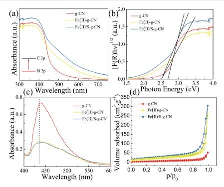
Fig. 5 UV-vis absorbance spectra (a), corresponding Kubelka-Munk plots (b), PL (c) and adsorption-desorption isothermal curve of N<sub>2</sub> (d) of the pure  $g-C_3N_4$  nanosheets and  $Fe(II)-g-C_3N_4$  and  $Fe(II)/S-g-C_3N_4$ .
