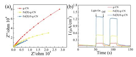
Fig. 6 EIS spectra (a), transient photocurrent response (b) of the pure,  $Fe(II)-g-C_3N_4$  and  $Fe(III)/S-g-C_3N_4$  catalysts.
