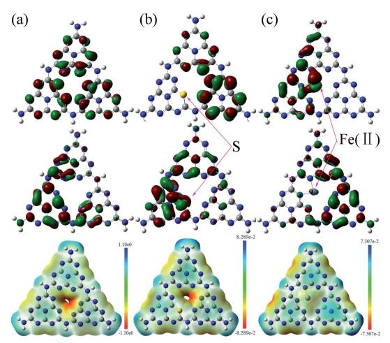
Fig. 9 Calculated HOMO (top), LUMO (middle) and surface electrostatic potential (bottom) of the pristine (a), S doped (b) and Fe(II) doped (c) g- $C_3N_4$  monolayer. The isosurface is taken at a value of 0.003 e bohr<sup>-3</sup>. Carbon atoms are in grey and nitrogen in blue.
