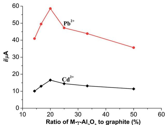
Fig. 4 Influences of different mass ratios (M- $\gamma$ -Al<sub>2</sub>O<sub>3</sub> to graphite powder) on the current responses of 10  $\mu\text{mol L}^{-1}$  Cd<sup>2+</sup> and 10  $\mu\text{mol L}^{-1}$  Pb<sup>2+</sup>. Supporting electrolyte: 0.1 mol L<sup>-1</sup> NaAc–HAc buffer solution (pH 4.5); accumulation potential: –1.0 V; accumulation time: 180 s; pulse amplitude: 0.05 V; pulse width: 0.05 s; pulse period: 0.2 s.
