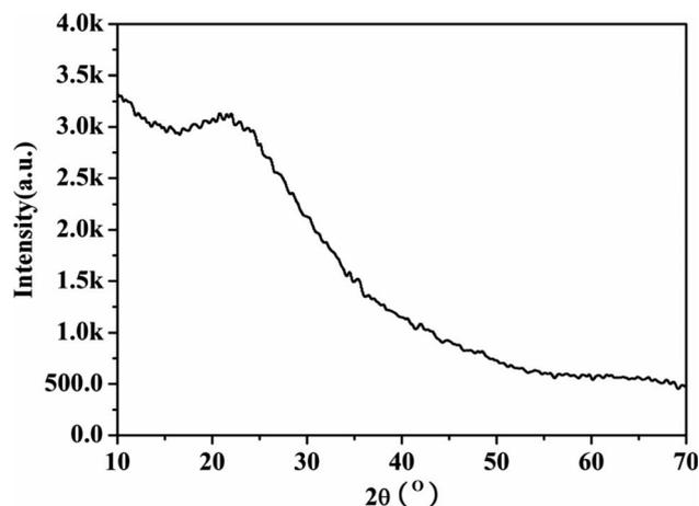
Fig. 1 The PXRD spectrum of the large surface area M- $\gamma$ -Al<sub>2</sub>O<sub>3</sub>.
