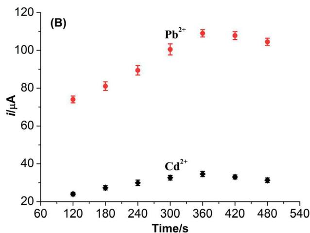
Fig. 8 (A) Influence of accumulation potential on the peak currents of  $\text{Pb}^{2+}$  and  $\text{Cd}^{2+}$ . (B) Influence of accumulation time on the peak currents of  $\text{Pb}^{2+}$  and  $\text{Cd}^{2+}$ .
