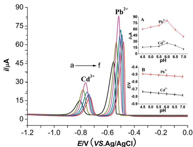
Fig. 7 Effect of different pH on  $10 \mu\text{mol L}^{-1} \text{Cd}^{2+}$  and  $10 \mu\text{mol L}^{-1} \text{Pb}^{2+}$  at a  $\text{M-Al}_2\text{O}_3$  modified carbon paste electrode. Inset (A): plots of  $i$  vs. pH for  $\text{Pb}^{2+}$  and  $\text{Cd}^{2+}$ , respectively. Inset (B): plots of  $i$  vs. pH for  $\text{Pb}^{2+}$  and  $\text{Cd}^{2+}$ , respectively. pH: a – 7.0, b – 6.5, c – 6.0, d – 5.5, e – 5.0, f – 4.5; other conditions are the same as Fig. 4.
