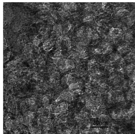
Fig. 3 The TEM image of the large surface area M- $\gamma$ -Al<sub>2</sub>O<sub>3</sub>.
