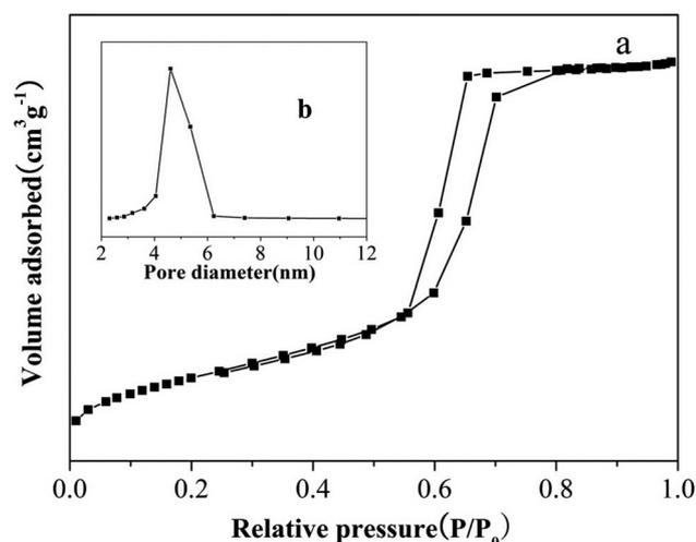
Fig. 2 (a) Nitrogen adsorption–desorption isotherm and (b) pore-size distribution of the large surface area M- $\gamma$ -Al<sub>2</sub>O<sub>3</sub>.
