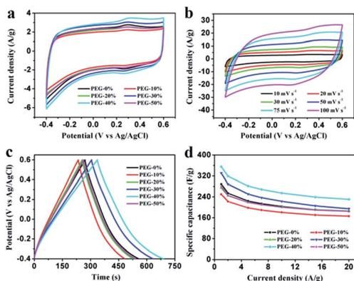
Fig. 6 Electrochemical performances of the PEG-*x*% materials based electrode measure in a three-electrode system in 1 M H<sub>2</sub>SO<sub>4</sub> aqueous electrolyte. (a) CV curves at a scan rate of 10 mV s<sup>-1</sup>; (b) CV curves of PEG-40% electrode material at different scan rates; (c) GCD curves at a current density of 1 A g<sup>-1</sup>; (d) specific capacitances at different current densities.
