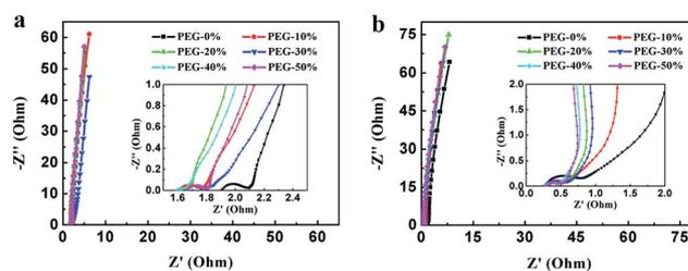
Fig. 8 Nyquist plots measured in 1 M H<sub>2</sub>SO<sub>4</sub> (a) and 2 M KOH (b). The inset shows a magnified view of the high frequency region of the impedance spectra.
