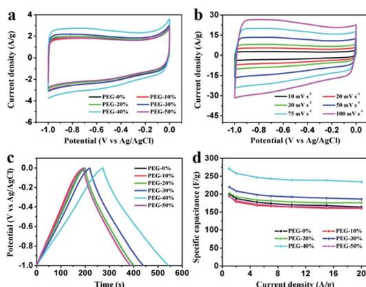
Fig. 7 Electrochemical performances of the PEG-*x*% materials based electrode measure in a three-electrode system in 2 M KOH aqueous electrolyte. (a) CV curves at a scan rate of 10 mV s<sup>-1</sup>; (b) CV curves of PEG-40% electrode material at different scan rates; (c) GCD curves at a current density of 1 A g<sup>-1</sup>; (d) specific capacitances at different current densities.
