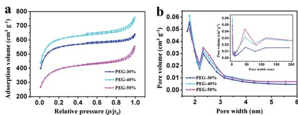
Fig. 5 (a) N<sub>2</sub> adsorption-desorption isotherms at 77 K and (b) PSD curves of PEG-30%, PEG-40% and PEG-50% samples.
