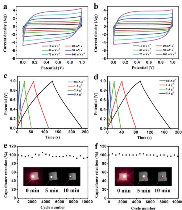
Fig. 9 Electrochemical performance of PEG-40% symmetrical supercapacitors in  $1 \text{ M H}_2\text{SO}_4$  and  $2 \text{ M KOH}$ , respectively. (a, b) CV curves at different scanning rates; (c, d) GCD curves at different current densities; (e, f) cycling stability at a  $1 \text{ A g}^{-1}$ .
