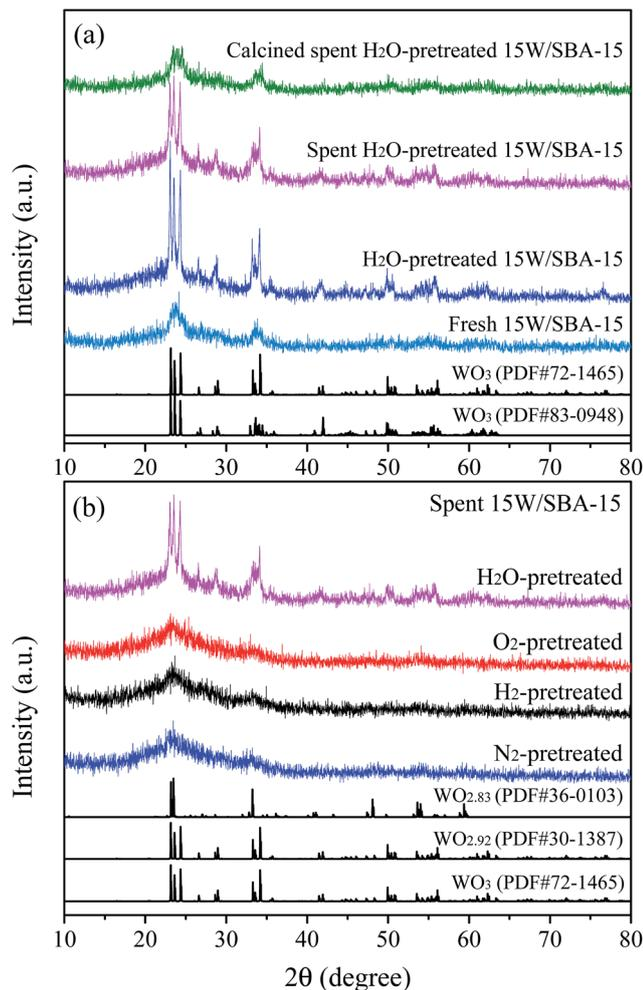
Fig. 9 XRD patterns of (a) fresh 15W/SBA-15, H<sub>2</sub>O-pretreated 15W/SBA-15, spent H<sub>2</sub>O-pretreated 15W/SBA-15, calcined spent H<sub>2</sub>O-pretreated 15W/SBA-15, and (b) spent 15W/SBA-15 catalysts pretreated in different gases (N<sub>2</sub>, H<sub>2</sub>, O<sub>2</sub> and H<sub>2</sub>O).
