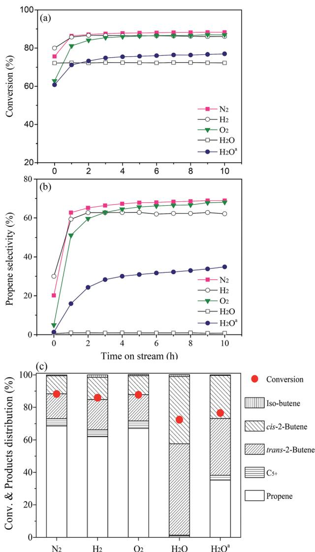
**Fig. 8** Time-dependence of 1-butene conversion (a), propene selectivity (b), and products distribution (c) over 15W/SBA-15 catalysts pretreated in different gases at the reaction conditions of 450 °C, 0.1 MPa, 0.5 g of catalyst weight, 1.8 h<sup>-1</sup> of WHSV, and an ethylene/1-butene molar ratio of 2. <sup>a</sup> Spent 15W/SBA-15 catalyst pretreated in H<sub>2</sub>O followed by calcination, and the obtained catalyst further treated in N<sub>2</sub> stream before reaction.
