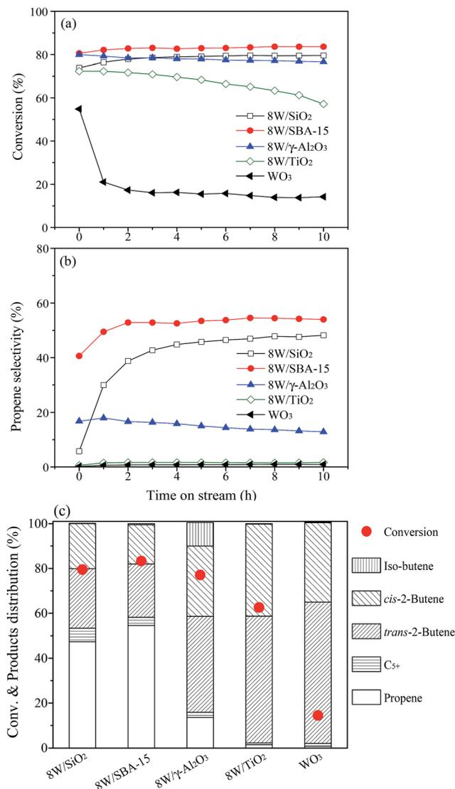
Fig. 2 Time-dependence of 1-butene conversion (a), propene selectivity (b), and products distribution (c) obtained over  $\text{WO}_3$  and various 8 wt% W-containing catalysts at the reaction conditions of 450 °C, 0.1 MPa, 0.5 g of catalyst weight, 1.8  $\text{h}^{-1}$  of WHSV, and an ethylene/1-butene molar ratio of 2.
