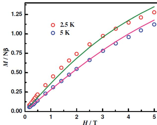
Fig. 10 Magnetization of  $\{[\text{Cu}^{\text{II}}\text{L}(\text{ClO}_4)]_2\text{Fe}^{\text{II}}(\text{CH}_3\text{OH})_2\}$  (**4**) at the indicated temperatures. The symbols are the experimental data, while the solid lines represent the fitted curves.
