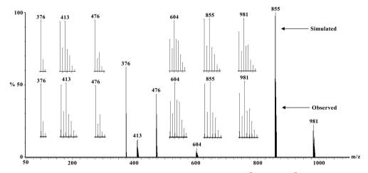
Fig. 6 Electrospray ionization mass spectrum in positive mode (ESI-MS positive) of [{Cu<sup>II</sup>L(ClO<sub>4</sub>)}<sub>2</sub>Mn<sup>II</sup>(CH<sub>3</sub>OH)<sub>2</sub>] (5) in acetonitrile, showing observed and simulated isotopic distribution patterns.
