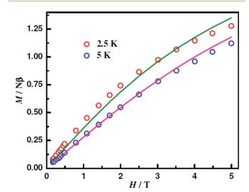
Fig. 10 Magnetization of  $[\{Cu^{II}L(ClO_4)\}_2Fe^{II}(CH_3OH)_2]$  (4) at the indicated temperatures. The symbols are the experimental data, while the solid lines represent the fitted curves.
