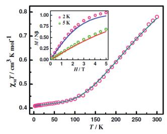
Fig. 7 Fitting of  $\chi_{M}T$  versus T of  $[\{Cu^{II}L(ClO_4)\}_2Cu^{II}(H_2O)]\cdot 2H_2O$  (1) between 2 and 300 K. The experimental data are shown in symbols and the lines correspond to the fitted values. The inset graph shows magnetization of  $[\{Cu^{II}L(ClO_4)\}_2Cu^{II}(H_2O)]\cdot 2H_2O$  (1) at the indicated temperatures. The symbols are the experimental data, while the solid lines represent the fitted curves.
