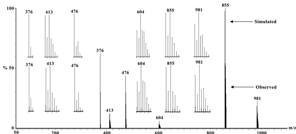
Fig. 6 Electrospray ionization mass spectrum in positive mode (ESI-MS positive) of  $[(\text{Cu}^{\text{II}}\text{L}(\text{ClO}_4))_2\text{Mn}^{\text{II}}(\text{CH}_3\text{OH})_2]$  (**5**) in acetonitrile, showing observed and simulated isotopic distribution patterns.
