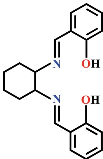
Scheme 1 Chemical structure of H<sub>2</sub>L.
