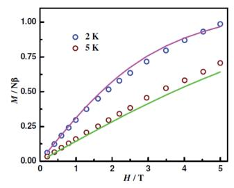
Fig. 9 Magnetization of [ $\{Cu^{II}L(CIO_4)\}\{Co^{II}(CH_3COCH_3),(H_2O)\}\}\{Cu^{II}L(CH_3COCH_3)\}\}CIO_4$  (3) at the indicated temperatures. The symbols are the experimental data, while the solid lines represent the fitted curves.
