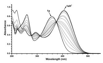
Fig. 3 UV/Vis absorption spectra resulting from protonation of PyDHA 1a ( $7.0 \times 10^{-5}$  mol  $L^{-1}$ ) with TFA in MeCN. The spectra presented are in the range of 0 equiv. TFA to 200 equiv. TFA. For full details of protonation, see ESI.†
