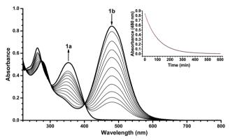
Fig. 1 UV/Vis absorption spectra recorded at 25 °C in MeCN. Top: Acquired during the ring-opening of Py-DHA **1a** to **1b**. Bottom: Acquired during the ring closure of **1b** to **1a**. Inset: Decay of VHF absorbance (at 480 nm) against time (min) (first-order kinetics).
