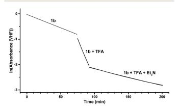
Fig. 4 Natural logarithm (In) of the VHF absorbance (at a wavelength of 480 nm for 1b and 1b + TFA + Et $_3$ N mixture and at 483 nm for 1b + TFA mixture) against time. The thermal heat release is activated by addition of TFA (steep slope) and the heat release is retarded again upon addition of Et $_3$ N.
