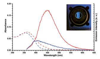
Fig. 7 UV/Vis absorption (broken line) and emission (full line) spectrum of 2a (blue) and 2aH+ (with 20 equiv. TFA; red) in abs. EtOH at 25 °C. Inset: Photo of the cuvette of 2aH<sup>+</sup> upon light irradiation (365 nm) inside the cryostat at -50 °C.
