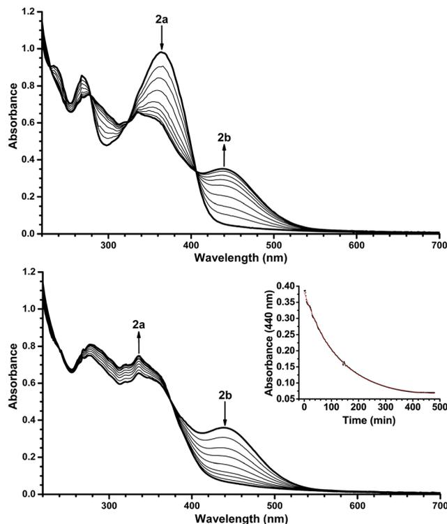
Fig. 5 UV/Vis absorption spectra recorded at  $-50\text{ }^{\circ}\text{C}$  in EtOH. Top: Acquired during the ring-opening of DHIQ-DHA **2a** to **2b**. Bottom: Acquired during the ring closure of **2b** to **2a**. Inset: Decay of VHF absorbance (440 nm) against time (min) (first-order kinetics).
