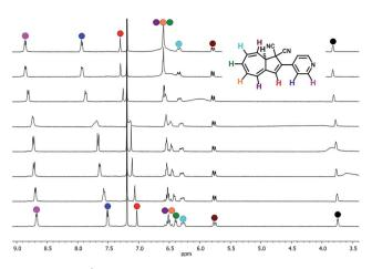
Fig. 2 Stacked  $^{1}$ H-NMR spectra recorded upon protonation of 1a (bottom) to  $1aH^{+}$  (top) with TFA in CDCl<sub>3</sub> (300 MHz); each spectrum corresponds to subsequent addition of 0.2 equiv. of TFA.
