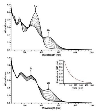
Fig. 5 UV/Vis absorption spectra recorded at -50 °C in EtOH. Top: Acquired during the ring-opening of DHIQ-DHA 2a to 2b. Bottom: Acquired during the ring closure of 2b to 2a. Inset: Decay of VHF absorbance (440 nm) against time (min) (first-order kinetics).
