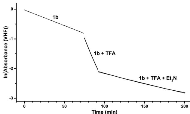
Fig. 4 Natural logarithm ( $\ln$ ) of the VHF absorbance (at a wavelength of 480 nm for **1b** and **1b + TFA + Et<sub>3</sub>N** mixture and at 483 nm for **1b + TFA** mixture) against time. The thermal heat release is activated by addition of TFA (steep slope) and the heat release is retarded again upon addition of  $\text{Et}_3\text{N}$ .
