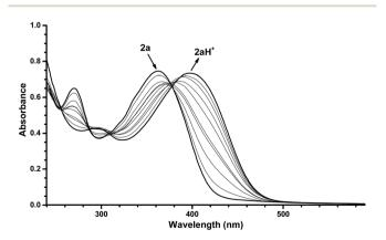
Fig. 6 UV/Vis absorption spectra resulting from protonation of DHIQ-DHA 2a (6.6  $\times$  10<sup>-5</sup> mol L<sup>-1</sup>) with TFA in EtOH. The spectra presented are in the range of 0 equiv. TFA to 400 equiv. TFA. For full details of protonation, see ESI.†
