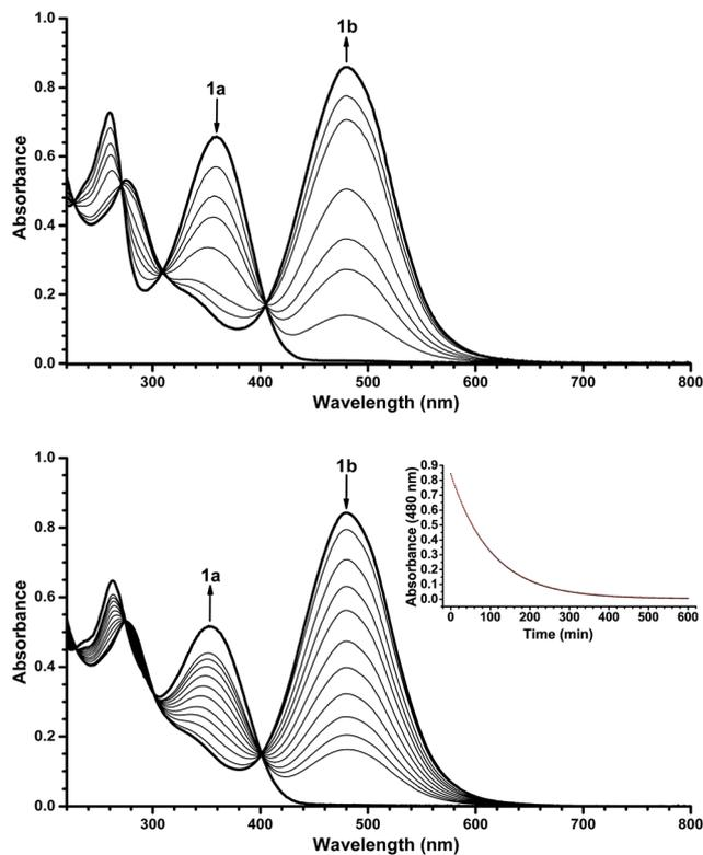
Fig. 1 UV/Vis absorption spectra recorded at 25 °C in MeCN. Top: Acquired during the ring-opening of Py-DHA **1a** to **1b**. Bottom: Acquired during the ring closure of **1b** to **1a**. Inset: Decay of VHF absorbance (at 480 nm) against time (min) (first-order kinetics).
