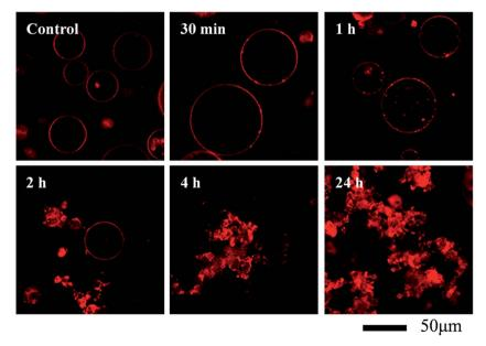
Fig. 3 Morphological changes of RhB-labeled GUVs<sup>+</sup> after exposure to 100 mg L<sup>-1</sup> C<sub>60</sub> NPs in 0.1 M glucose.
