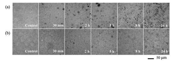
Fig. 2 Bright field images of GUVs<sup>+</sup> (a) and GUVs<sup>-</sup> (b) after exposure to 100 mg L<sup>-1</sup>  $C_{60}$  NPs in 0.1 M glucose.
