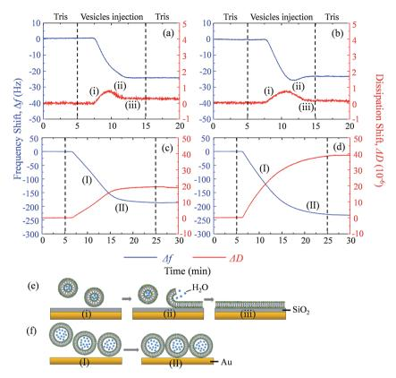
Fig. 4 Frequency shifts ( $\Delta f$ , blue) and dissipation shifts ( $\Delta D$ , red) during the formation of SLB<sup>+</sup> (a), SLB<sup>-</sup> (b), SUV<sup>+</sup> layer (c) and SUV<sup>-</sup> layer (d) at pH 7.0. The formation of SLB on a silica sensor (e) and the formation of a SUV layer on a gold sensor (f) are illustrated.
