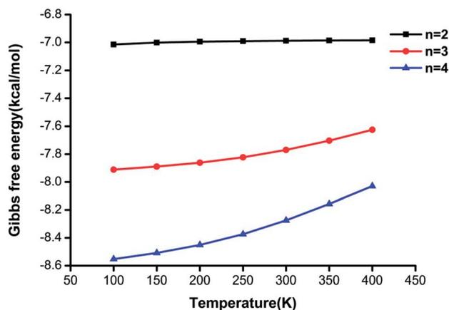
**Fig. 6** Changes in the Gibbs free energy (in  $\text{kcal mol}^{-1}$ ) of the global minimum structures of the  $(\text{H}_2\text{C}_2\text{O}_4)(\text{CH}_3\text{NH}_2)_n$  ( $n = 2-4$ ) clusters as a function of temperature at the PW91PW91/6-311++G(3df,3pd) level of theory.
