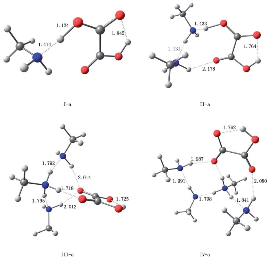
Fig. 2 Lowest-energy structures of the  $(\text{H}_2\text{C}_2\text{O}_4)(\text{CH}_3\text{NH}_2)_n$  ( $n = 1-4$ ) clusters at the PW91PW91/6-311++G(3df,3pd) level of theory ordered according to the state of association (I, II, III, IV). The intramolecular and intermolecular interaction distances are given.
