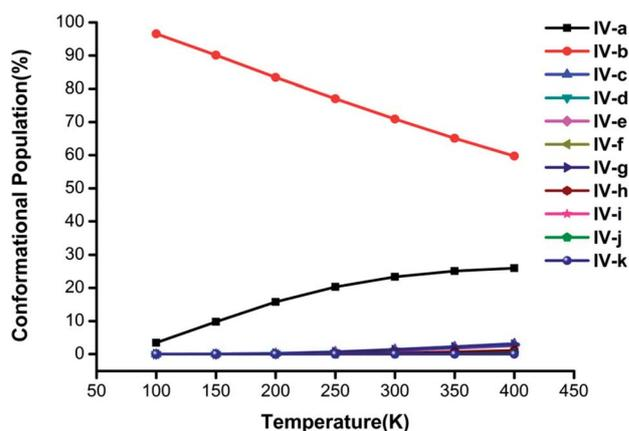
**Fig. 5** Changes in the conformational populations of the low-energy isomers of (H<sub>2</sub>C<sub>2</sub>O<sub>4</sub>)(CH<sub>3</sub>NH<sub>2</sub>)<sub>4</sub> as a function of temperature.
