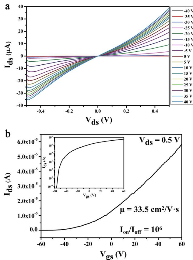
Fig. 3 The basic electrical characterization of the MoS<sub>2</sub> FET. (a) Output characteristic curve of the device, drain current ( $I_{ds}$ ) as a function of drain voltage ( $V_{ds}$ ) with the back gate voltage ( $V_{gs}$ ) varying from  $-40$  to  $40$  V, in a step of  $5$  V. (b) Transfer characteristic curve of the device,  $I_{ds}$  as a function of  $V_{gs}$  with the  $V_{ds}$  of  $0.5$  V. Inset, the logarithmic image of transfer characteristic curve ( $I_{ds}$ – $V_{gs}$ ).
