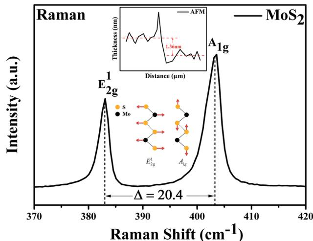
Fig. 2 Raman spectrum of the channel material. The number of layers of the MoS<sub>2</sub> nanosheet we prepared can be confirmed as bilayer. Inset, the height gradient between the channel material and the underlying substrate was tested by the AFM, the thickness of the MoS<sub>2</sub> channel material is 1.36 nm.
