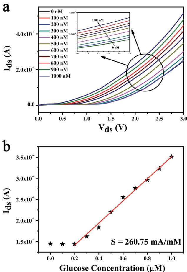
Fig. 5  $\text{MoS}_2$  FET sensor for ultra low concentration glucose sensing. (a) The detection limit of the biosensor based on  $\text{MoS}_2$  FET observed by the output characteristic curve is 300 nM. (b) Drain current as a function of glucose concentration which ranges from 0 to 1  $\mu\text{M}$  at  $V_{\text{gs}}$  of 0.5 V and  $V_{\text{ds}}$  of 2.5 V. By calculation, the sensitivity of our biosensor has been achieved as high as 260.75  $\text{mA mM}^{-1}$ .
