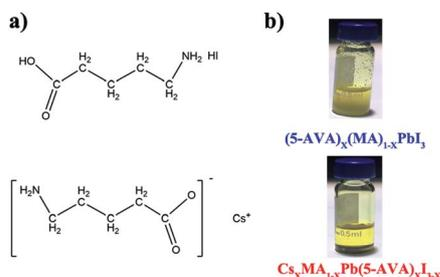
Fig. 1 (a) The molecular structure of (5-AVA) iodide and Cs-(5-AVA) acetate. (b) Optical images of (5-AVA)<sub>x</sub>(MA)<sub>1-x</sub>PbI<sub>3</sub> and Cs<sub>x</sub>MA<sub>1-x</sub>Pb(5-AVA)<sub>x</sub>I<sub>3-x</sub> perovskite solution at room temperature.
