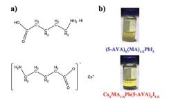
Fig. 1 (a) The molecular structure of (5-AVA) iodide and Cs-(5-AVA) acetate. (b) Optical images of  $(5-AVA)_x(MA)_{1-x}PbI_3$  and  $Cs_xMA_{1-x}Pb(5-x)$  $AVA)_xI_{3-x}$  perovskite solution at room temperature.
