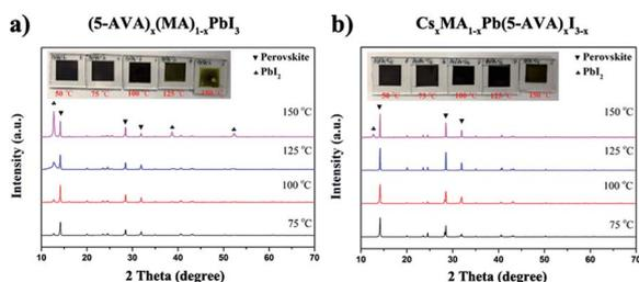
Fig. 5 XRD patterns and optical images (inset) of (a)  $(5\text{-AVA})_x(\text{MA})_{1-x}\text{PbI}_3$  and (b)  $\text{Cs}_x\text{MA}_{1-x}\text{Pb}(5\text{-AVA})_x\text{I}_{3-x}$  perovskite films exposed on a hot plate to various temperatures each for 24 h.
