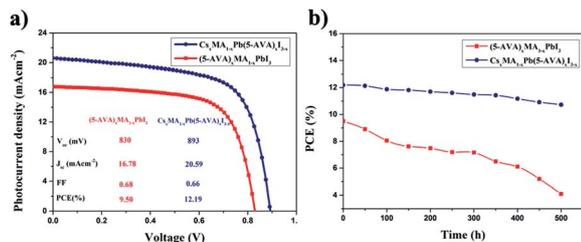
Fig. 4 (a)  $J$ - $V$  curves of the carbon-based PSCs with the  $(5\text{-AVA})_x(\text{MA})_{1-x}\text{PbI}_3$  and  $\text{Cs}_x\text{MA}_{1-x}\text{Pb}(5\text{-AVA})_x\text{I}_{3-x}$  perovskites. (b) Long-term stability of the carbon-based PSCs stored at 100 °C in glove box.
