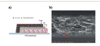
Fig. 3 (a) Schematic structure of the carbon-based PSC. (b) SEM image from a cross-section of the carbon-based PSC.
