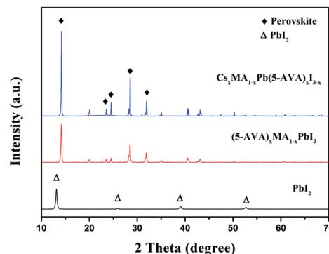
Fig. 2 XRD patterns of the PbI<sub>2</sub>, (5-AVA)<sub>x</sub>(MA)<sub>1-x</sub>PbI<sub>3</sub> and Cs<sub>x</sub>MA<sub>1-x</sub>Pb(5-AVA)<sub>x</sub>I<sub>3-x</sub> films on glass substrates.
