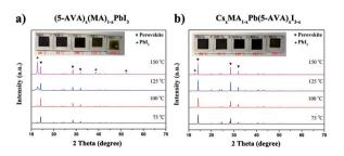
Fig. 5 XRD patterns and optical images (inset) of (a)  $(5-AVA)_x(MA)_{1-x}PbI_3$  and (b)  $Cs_xMA_{1-x}Pb(5-AVA)_xI_{3-x}$  perovskite films exposed on a hot plate to various temperatures each for 24 h.
