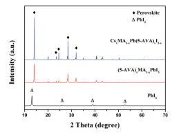
Fig. 2 XRD patterns of the PbI<sub>2</sub>,  $(5-AVA)_x(MA)_{1-x}PbI_3$  and  $Cs_xMA_{1-x}-$ Pb(5-AVA)<sub>x</sub> $I_{3-x}$  films on glass substrates.
