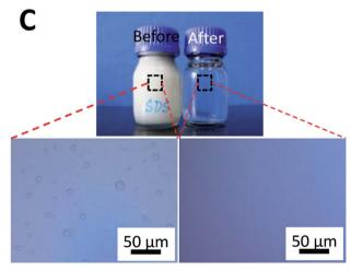
Fig. 2 (A) SEM image of the PEM-coated polycarbonate membrane. (B) The filtration flux represented by volume of the filtrate collected in a 10 min cycle as a function of the cycle number for the virgin membrane and membranes coated with PSS-capped PEM $_n$  with n=1-4 in separation of the SDS-stabilized emulsion. (C) Photograph of the SDS-stabilized oil-in-water emulsion, before and after filtration, and optical microscopy images of the emulsion feed and the filtrate.
