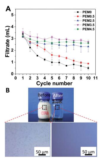
Fig. 3 (A) The filtration flux represented by volume of the filtrate collected in a 10 min cycle as a function of the cycle number for the virgin membrane and membranes coated with PDDA-capped PEM $_n$  with n=0.5, 2.5, 3.5 and 4.5, respectively, in separation of the CTAB-stabilized emulsion. (B) Photograph of the CTAB-stabilized oil-inwater emulsion, before and after filtration, and optical microscopy images of the emulsion feed and the filtrate.
