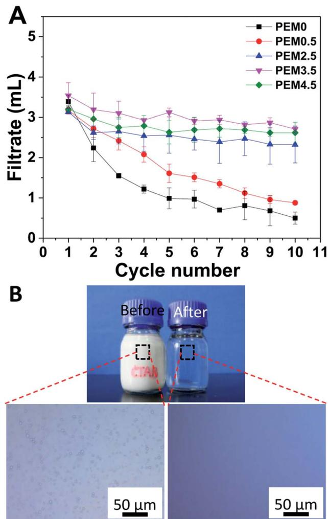
Fig. 3 (A) The filtration flux represented by volume of the filtrate collected in a 10 min cycle as a function of the cycle number for the virgin membrane and membranes coated with PDPA-capped PEM<sub>n</sub> with  $n = 0.5, 2.5, 3.5$  and  $4.5$ , respectively, in separation of the CTAB-stabilized emulsion. (B) Photograph of the CTAB-stabilized oil-in-water emulsion, before and after filtration, and optical microscopy images of the emulsion feed and the filtrate.
