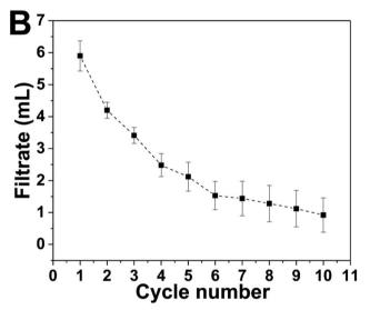
Fig. 1 (A) SEM image of a virgin hydrophilic polycarbonate membrane. The inset shows a magnified view of the perpendicular pores with a diameter of *ca.* 200 nm in the membrane. (B) The filtration flux represented by volume of the filtrate collected in a 10 min cycle as a function of the cycle number for the virgin membrane.
