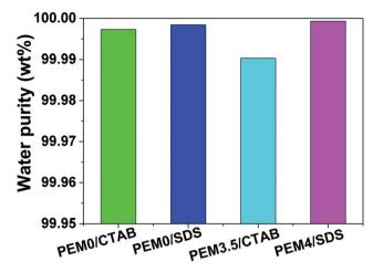
Fig. 4 Purity of filtrate separated by different membranes.
