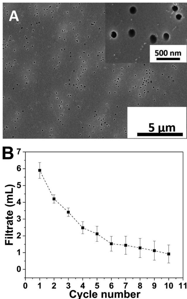
**Fig. 1** (A) SEM image of a virgin hydrophilic polycarbonate membrane. The inset shows a magnified view of the perpendicular pores with a diameter of ca. 200 nm in the membrane. (B) The filtration flux represented by volume of the filtrate collected in a 10 min cycle as a function of the cycle number for the virgin membrane.
