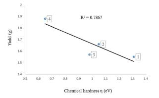
Fig. 6 A graph of chemical hardness against yield of oligomers produced using complexes 1–4.
