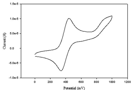
Fig. 3 Cyclic voltammogram of compound L2 in DMF, [<sup>t</sup>BuN][BF<sub>4</sub>] as supporting electrolyte, Ag/AgCl as reference electrode, platinum wire as counter electrode, glassy carbon as working electrode, scan rate of 100 mV s<sup>-1</sup>, temperature 25 °C.
