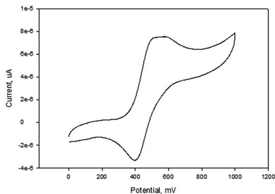
Fig. 4 Cyclic voltammogram of complex 1 in DMF, [<sup>t</sup>BuN][BF<sub>4</sub>] as supporting electrolyte, Ag/AgCl as reference electrode, platinum wire as counter electrode, glassy carbon as working electrode, scan rate of 100 mV s<sup>-1</sup>, temperature = 25 °C.
