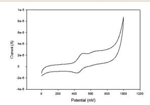
Fig. 5 Cyclic voltammogram of complex 6 in DMF, [<sup>t</sup>BuN][BF<sub>4</sub>] as supporting electrolyte, Ag/AgCl as reference electrode, platinum wire as counter electrode, glassy carbon as working electrode, scan rate of 100 mV s<sup>-1</sup>, temperature 25 °C
