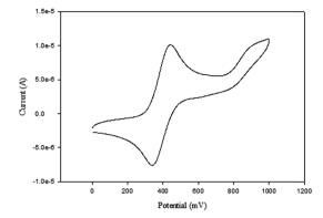
Fig. 3 Cyclic voltammogram of compound L2 in DMF, [tBuN][BF4] as supporting electrolyte, Ag/AgCl as reference electrode, platinum wire as counter electrode, glassy carbon as working electrode, scan rate of 100 mV s<sup>-1</sup>, temperature 25 °C.
