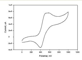
Fig. 4 Cyclic voltammogram of complex 1 in DMF, [tBuN][BF4] as supporting electrolyte, Ag/AgCl as reference electrode, platinum wire as counter electrode, glassy carbon as working electrode, scan rate of 100 mV s<sup>-1</sup>, temperature =  $25 \, ^{\circ}$ C.
