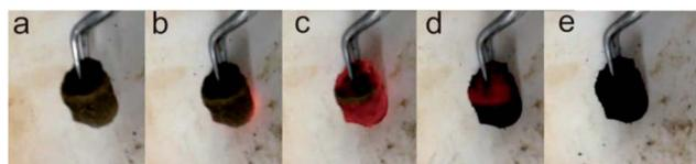
**Fig. 2** Optical photos of the combustion process of GOA. (a) The brown columnar GOA before contacting the hot plate, (b)–(d) the process of combustion in less than 0.3 s, and (e) the black fluffy P-RGO was obtained after all.
