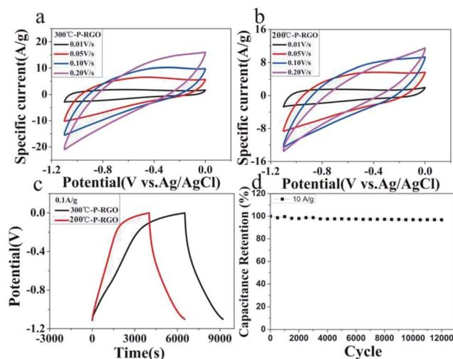
Fig. 7 Electrochemical tests of P-RGO based supercapacitors: (a) CV graph of 300-P-RGO, (b) CV graph of 200-P-RGO, (c) GCD graph of 300-P-RGO and 200-P-RGO at the current density 0.1 A g<sup>−1</sup>, and (d) the capacitance retention rates for various cycle numbers up to 12 000 cycles at the current density 10A g<sup>−1</sup> by the GCD test.
