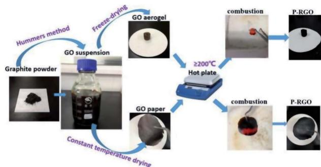
**Fig. 1** The schematic illustration displays the combustion method for preparing P-RGO. Starting from graphite powder, *via* Hummers method, GO suspension was then obtained. By way of freeze-drying/constant temperature drying, GO aerogel/GO paper was produced. Then, GO aerogel/GO paper combusted through the process of the thermal treatment, and P-RGO was obtained.
