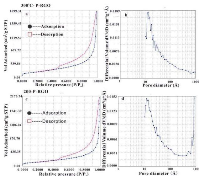
Fig. 5 (a)  $N_2$  physical adsorption isotherm and (b) BJH adsorption pore size distribution of the 300-P-RGO. (c)  $N_2$  physical adsorption isotherm and (d) BJH adsorption pore size distribution of the 200-P-RGO.
