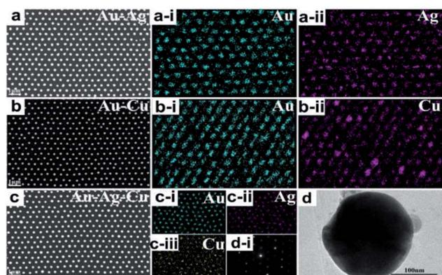
Fig. 2 SEM plan-view images and corresponding EDS elemental distributing map of alloyed NPs arrays templated by colloidal monolayer with periodic length of 500 nm: Au–Ag (a), Au–Cu (b), Au–Ag–Cu (c) alloyed NPs arrays. (d) TEM image of a single isolate Au–Ag–Cu NP, (d–i) Electron diffraction pattern of the single isolate Au–Ag–Cu NP.
