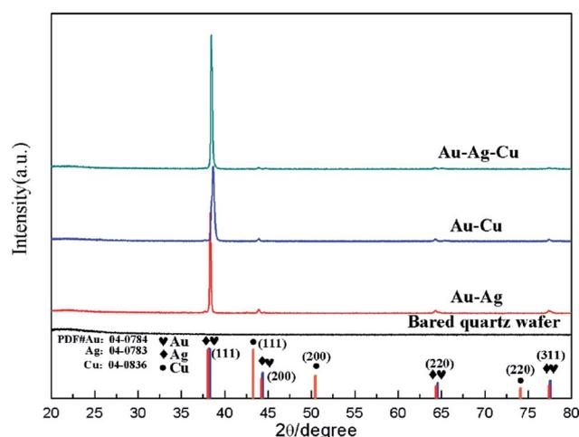
Fig. 3 XRD pattern of obtained periodic alloyed NPs arrays by colloidal monolayer crystal with periodicity of 500 nm.
