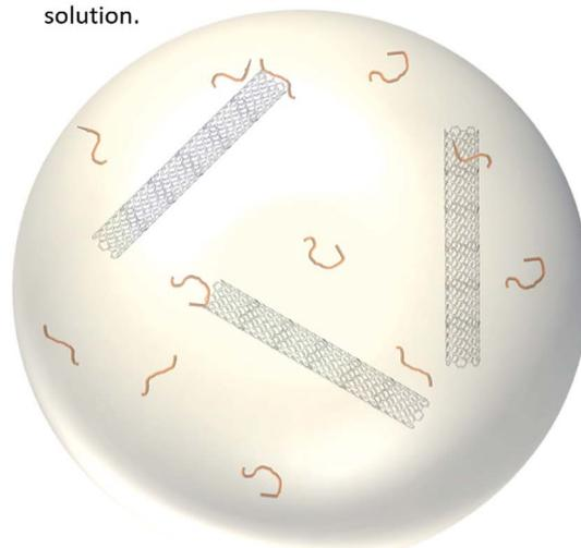
Surfactant present at ≥ 1.5 mg/ml- Individual CNTs contained in nanoscale individual droplets of PCL solution.
