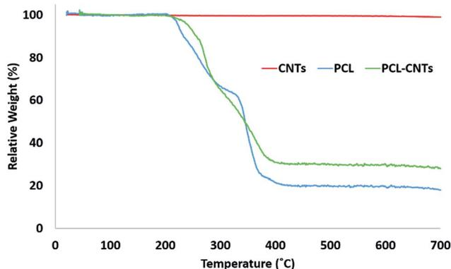
**Fig. 6** Analysis of the PCL-CNT (93% PCL, 7% CNTs by mass) nanocomposite and its constituents by TGA. The concentrations used during preparation were 10 mg mL<sup>-1</sup> of PCL and 1.5 mg mL<sup>-1</sup> SDS for PCL; 10 mg mL<sup>-1</sup> of PCL, 1.5 mg mL<sup>-1</sup> SDS and 0.9 mg mL<sup>-1</sup> CNTs for PCL-CNTs. CNTs consists of 0.9 mg mL<sup>-1</sup> CNTs alone.
