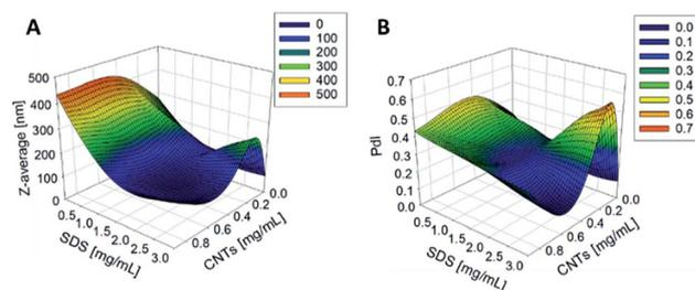
Fig. 2 The effect of changing the concentration of CNTs and SDS on the Z-average diameter (A) and the PdI (B) of the resulting nanoparticles as measured by DLS. The concentration of PCL was  $6 \text{ mg mL}^{-1}$ .
