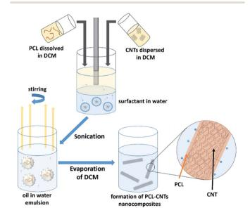
Fig. 1 Scheme for the preparation of PCL-CNTs nanocomposites by an oil-in water emulsion solvent evaporation method. The solution of PCL and dispersion of CNTs (both in DCM) was emulsified in an aqueous surfactant solution. The resulting emulsion was kept stirring until the DCM had evaporated resulting in PCL-CNTs nanocomposites.
