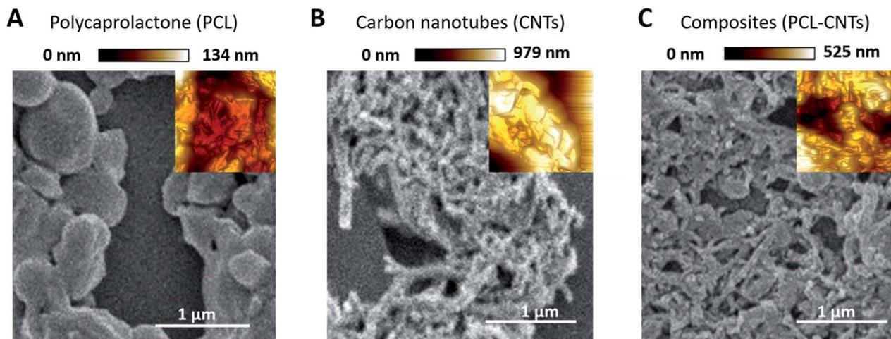
**Fig. 5** Analysis of the PCL, CNT and PCL-CNT (93% PCL, 7% CNTs by mass) nanocomposites by SEM and AFM (inset): (A) PCL alone, (B) CNTs and (C) PCL-CNTs composites. The AFM images are based on the peak force error measurements. The AFM images were not obtained from the same region shown in the SEM image, but have been inset so as to assist direct comparison with the morphologies revealed both techniques at the same scale. The scale bar applies to both the SEM images and inset AFM images.
