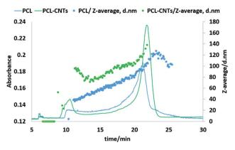
Fig. 7 Fractogram of PCL and PCL-CNTs (93% PCL, 7% CNTs by mass) obtained from asymmetric flow field flow fractionation coupled online with UV-VIS detector. Hydrodynamic diameters were obtained from DLS coupled online.
