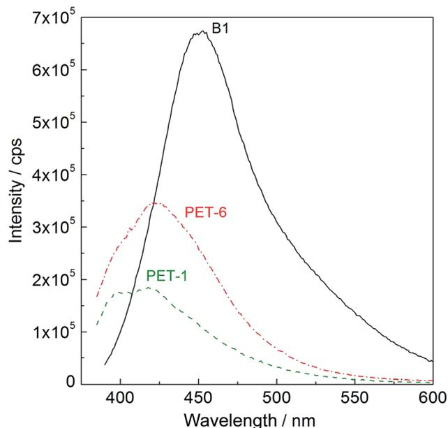
Fig. 3 UV-vis spectra (at 380 nm) of the original borane compound *anti*-B<sub>18</sub>H<sub>22</sub> (B1, black solid line), pristine PET foil (PET-1, green dashed line) and PET foil after activation with piranha solution and grafting with cysteamine and subsequently with B1 (PET-6, red dashed-dot line).
