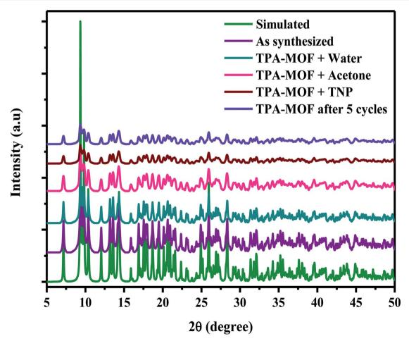
Fig. 6 PXRD spectra obtained after immersion in H<sub>2</sub>O (4 days), acetone, and TNP for 72 h and recycled sample after five cycles.
