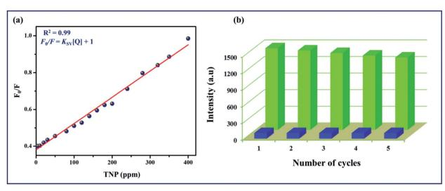
Fig. 5 (a) Stern-Volmer plot of  $F_0/F$  vs. TNP (ppm) concentration in aqueous solution for TPA-MOF, (b) quenching and reproducibility test for TPA-MOF (initial fluorescence intensity, green; intensity after quenching (400 ppm TNP), blue).
