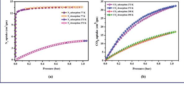
Fig. 2 Gas adsorption isotherms of TPA-MOF: (a) N<sub>2</sub> adsorption and desorption at 77 K and 273 K, (b) CO<sub>2</sub> adsorption and desorption at 273 K and 298 K.
