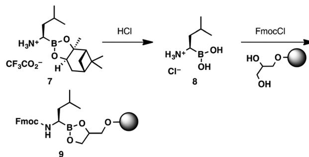
Scheme 3 2-Step protocol for loading boroleucine onto a 1-glycerol polystyrene resin.
