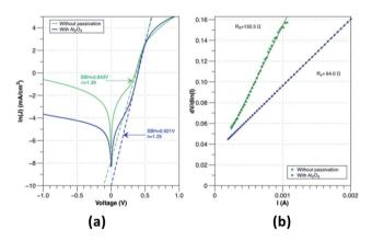
Fig. 5 (a) Dark J-V characteristics of Gr/Si solar cells with and without  $Al_2O_3$  interfacial layer. Inset shows the corresponding  $\ln J-V$  curves. (b) Plots of  $dV/d\ln(I)$  versus I for Gr/Si solar cells with and without  $Al_2O_3$  interfacial layer.
