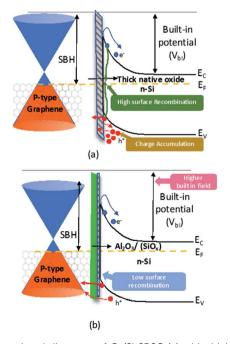
Fig. 6 Energy band diagrams of Gr/Si SBSC (a) with thick interfacial layer (b) with  $Al_2O_3/n$ ative oxide interfacial layers.
