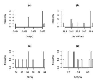
Fig. 4 Histogram of (a) open circuit voltage (b) short circuit current (c) fill factor (d) power conversion efficiency for Gr/Si solar cells with  $Al_2O_3$  interfacial layer.
