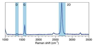
Fig. 1 Raman spectrum of synthesized graphene.<sup>28</sup>
