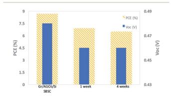
Fig. 7 Variation of PCE and  $V_{\rm oc}$  of Gr/Si with  $Al_2O_3$  interfacial layer over time
