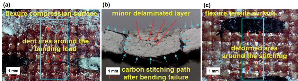
Fig. 13 Warp directional flexure failure in PAN carbon nanostitched *p*-aramid/phenolic MWCNT composites. (a) Stitched/nano top face (TB-CS-N); (b) stitched/nano cross-section (TB-CS-N); (c) stitched/nano bottom face (TB-CS-N) (optical microscope, magnification  $\times 6.7$ ).
