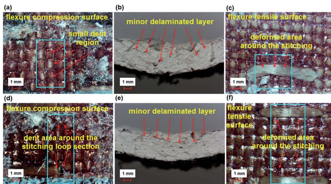
Fig. 12 Warp directional flexure failure in various multistitched 3D *p*-aramid/phenolic MWCNT composites. (a) Stitched top face (TB-TS); (b) stitched cross-section (TB-TS); (c) stitched bottom face (TB-TS); (d) stitched/nano top face (TB-TS-N); (e) stitched/nano cross-section (TB-TS-N) and (f) stitched/nano bottom face (TB-TS-N) (optical microscope, magnification  $\times 6.7$ ).
