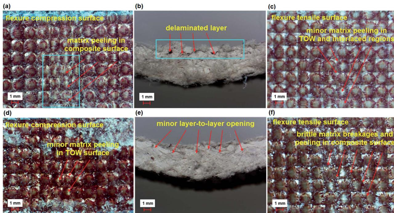
Fig. 11 Warp directional flexure failure in various multistitched 3D *p*-aramid/phenolic MWCNT composites. (a) Base top face (TBU); (b) base cross-section (TBU); (c) base bottom face (TBU); (d) base/nano top face (TBU-N); (e) base/nano cross-section (TBU-N) and (f) base/nano bottom face (TBU-N) (optical microscope, magnification  $\times 6.7$ ).
