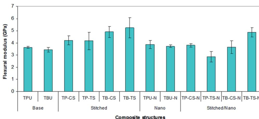
Fig. 10 Flexure modulus of various developed *p*-aramid/phenolic MWCNT composites.
