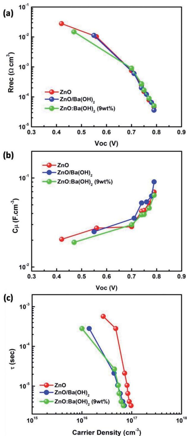
Fig. 6 (a) Recombination resistance ( $R_{rec}$ ) as a function of  $V_{oc}$  (b) chemical capacitance ( $C_{\mu}$ ) as a function of  $V_{oc}$  (c) carrier lifetime as a function of the photo-generated carrier density for PTB7-Th:PCBM OSCs with ZnO, ZnO/Ba(OH)<sub>2</sub> and ZnO:Ba(OH)<sub>2</sub> nanocomposite as ETLs.
