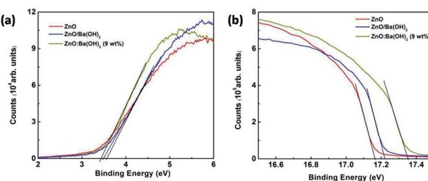
Fig. 5 UPS spectra of ZnO, ZnO/Ba(OH)<sub>2</sub> and ZnO:Ba(OH)<sub>2</sub> (9 wt%) nanocomposite thin films deposited on ITO coated glass substrates (a) valence band region (b) cut-off region.
