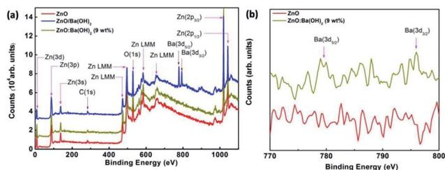
Fig. 4 (a) XPS Survey scan spectra of ZnO, ZnO/Ba(OH)<sub>2</sub> and ZnO:Ba(OH)<sub>2</sub> (9 wt%) nanocomposite thin films deposited on ITO coated glass substrates. (b) XPS core level spectra of ZnO and ZnO:Ba(OH)<sub>2</sub> (9 wt%) nanocomposite.
