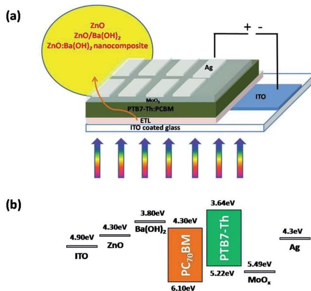
Fig. 1 (a) Schematic of PTB7-Th:PCBM OSCs in an inverted geometry with ZnO, ZnO/Ba(OH)<sub>2</sub> and ZnO:Ba(OH)<sub>2</sub> nanocomposite as ETLs (b) energy levels of materials used in the solar cell device.
