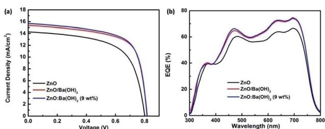
Fig. 2 (a)  $J$ – $V$  characteristics under illumination (AM 1.5 G, one sun) and (b) EQE spectra of devices with ZnO, ZnO/Ba(OH)<sub>2</sub> and ZnO:Ba(OH)<sub>2</sub> nanocomposite as an ETLs.
