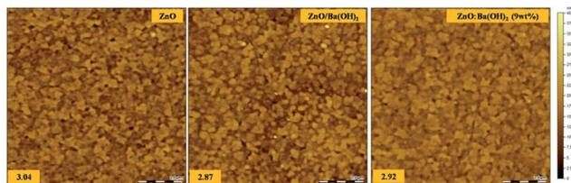
Fig. 3 Atomic Force Microscopy (AFM) images of ZnO, ZnO/Ba(OH)<sub>2</sub> and ZnO:Ba(OH)<sub>2</sub> (9 wt%) nanocomposite thin films deposited on ITO coated glass substrates.
