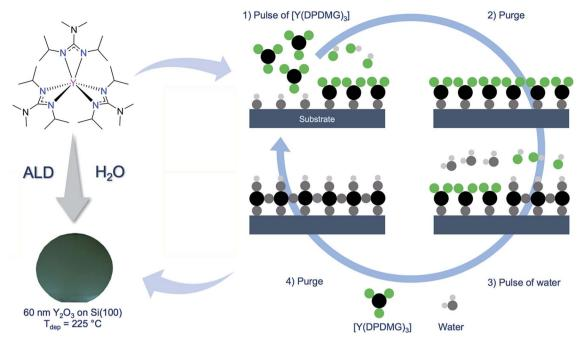
Scheme 1 Molecular structure of [Y(DPDMG)<sub>3</sub>]<sup>24</sup> (top-left). Highlighted are the six reactive Y-N bonds. (Bottom-left) A photograph of a 50 nm thick Y<sub>2</sub>O<sub>3</sub> thin film grown on 2-inch Si(100) wafer at 225 °C. (Right) A typical schematic representation of an ALD cycle involving the two highlighted precursors.
