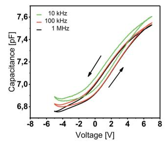
Fig. 5 Capacitance-voltage curves of Y<sub>2</sub>O<sub>3</sub> based MIS capacitors for f = 10 kHz, 100 kHz and 1 MHz. The 20 nm  $Y_2O_3$  thin film was deposited at 200 °C.
