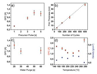
Fig. 1 (a) Precursor saturation studies by the variation of the  $[Y(DPDMG)_3]$  pulse length at 225 °C on Si(100). (b) Film thickness versus number of applied cycles. (c) GPC variation with water purge time at 225 °C on Si(100). (d) GPC and thin film density as a function of deposition temperature.
