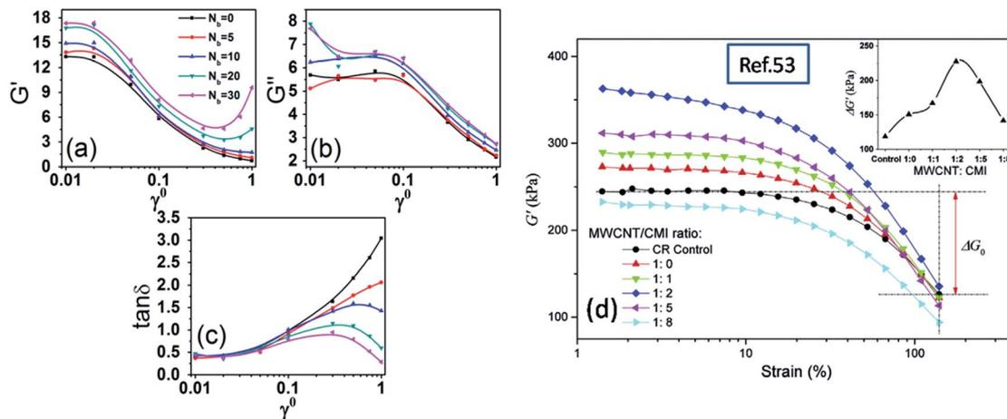
Fig. 2 (a) Storage modulus  $G'$ , (b) loss modulus  $G''$ , and (c) loss factor  $\tan \delta$ , as a function of shear strain amplitude for the systems with different polymer-particle chemical coupling on temperature at 1.0 and frequency at  $0.01\tau^{-1}$ . (d) Strain dependence of  $G'$  for CR/m-MWCNT composites with different MWCNT/CMI ratios (ref. 53).
