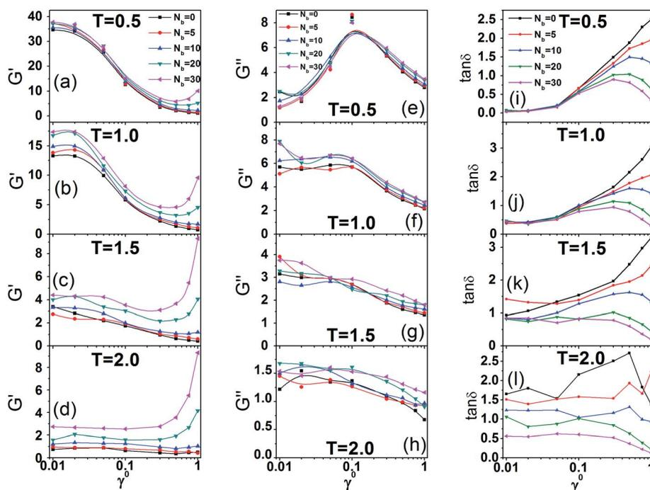
Fig. 3 (a–d) Storage modulus  $G'$ , (e–h) loss modulus  $G''$ , (i–l) loss factor, as a function of shear strain amplitude with various chemical coupling at different temperatures.
