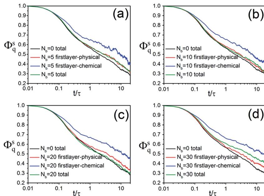
Fig. 10 Incoherent intermediate dynamic structure functions ( $\Phi_q^S$ ) of the polymers with or without chemical coupling located in the first polymer layer and NPs at  $\epsilon_{np} = 8.0$ . (a)  $N_b = 5$ , (b)  $N_b = 10$ , (c)  $N_b = 20$ , and (d)  $N_b = 30$ .
