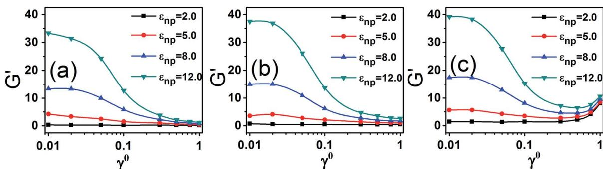
Fig. 5 Storage modulus  $G'$  as a function of shear strain amplitude with various interfacial physical interaction between NPs and polymers ( $\varepsilon_{np}$ ) in systems with different chemical coupling, (a)  $N_b = 0$ , (b)  $N_b = 10$ , and (c)  $N_b = 30$ .
