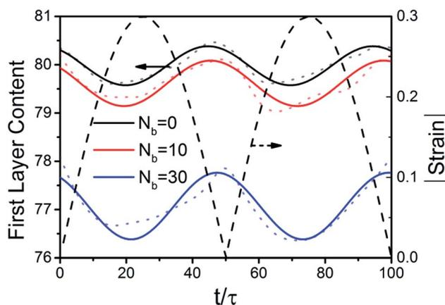
Fig. 9 Plot of the first layer content with respect to the oscillatory shear with the amplitude of 30% at  $\epsilon_{np} = 8.0$ . The periodic dash line represents the shear strain with respect to the time. The solid lines are the fitting curves according to the dot lines which represent the original data.
