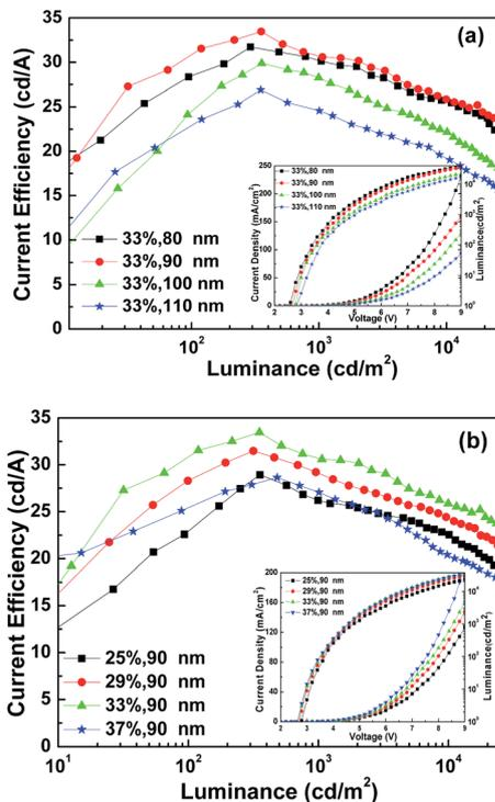
Fig. 8 (a) CE–L characteristics of devices Cl–ITO (o-DCB, UV 5 min)/TPBi:Ir(ppy)<sub>3</sub> (33%, Y nm, Y = 80, 90, 100, 110 nm)/LiF (0.7 nm)/Al (150 nm). The inset gives the J–L–V of the devices. (b) CE–L characteristics of devices Cl–ITO (o-DCB, UV 5 min)/TPBi:Ir(ppy)<sub>3</sub> (X%, 90 nm, X = 25, 29, 33, 37%)/LiF (0.7 nm)/Al (150 nm). The inset gives the J–L–V of the devices.
