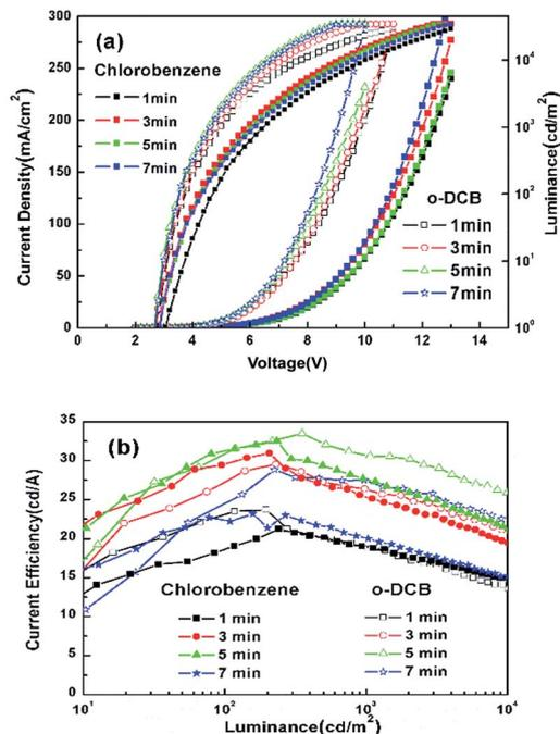
Fig. 5 (a) *J-V-L* and (b) *CE-L* characteristics of devices with ITO treated by *o*-DCB and chlorobenzene.
