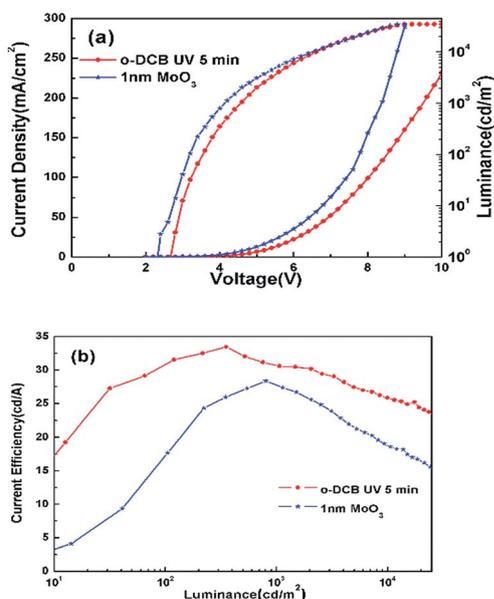
Fig. 9 (a)  $J$ – $V$ – $L$  and (b) CE–L characteristics of the device with ITO treated by o-DCB and the device with 1 nm MoO<sub>3</sub> as the ITO modified layer.
