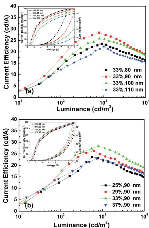
Fig. 3 (a) *CE*–*L* characteristics of the devices ITO/MoO<sub>3</sub> (1 nm)/TPBi:Ir(ppy)<sub>3</sub> (33%, Y nm, Y = 80, 90, 100, 110 nm)/LiF (0.7 nm)/Al (150 nm). The inset gives the *J*–*L*–*V* of the devices. (b) *JCE*–*L* characteristics of the devices ITO/MoO<sub>3</sub> (1 nm)/TPBi:Ir(ppy)<sub>3</sub> (X%, 90 nm, X = 25, 29, 33, 37%)/LiF (0.7 nm)/Al (150 nm). The inset gives the *J*–*L*–*V* of the devices.
