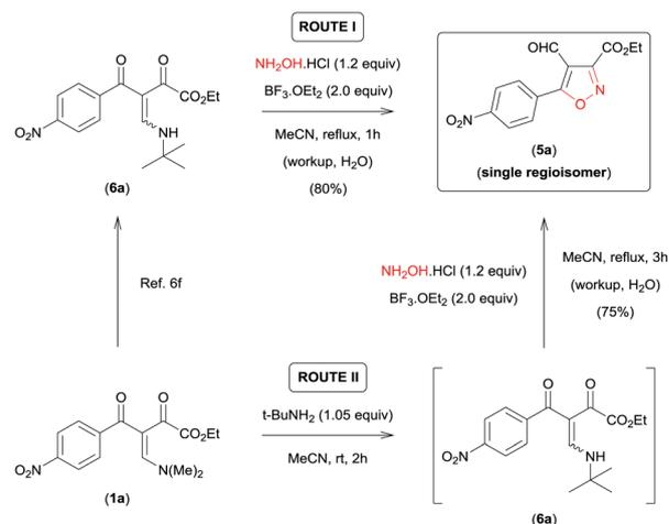
Scheme 2 ROUTE I – Synthesis of 3,5-disubstituted 4-formyl-isoxazol **5a** from  $\beta$ -enamino diketone **6a**; ROUTE II – sequential one-pot procedure to obtain **5a** from  $\beta$ -enamino diketone **1a**.
