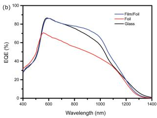
Fig. 4 (a) JV curves and (b) EQE response of solar cells on rigid and flexible substrates.
