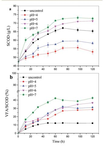
Fig. 2 Soluble chemical oxygen demand (SCOD) concentrations and the percentage of volatile fatty acid (VFA)/SCOD at various pH values and 100 g TS/L.
