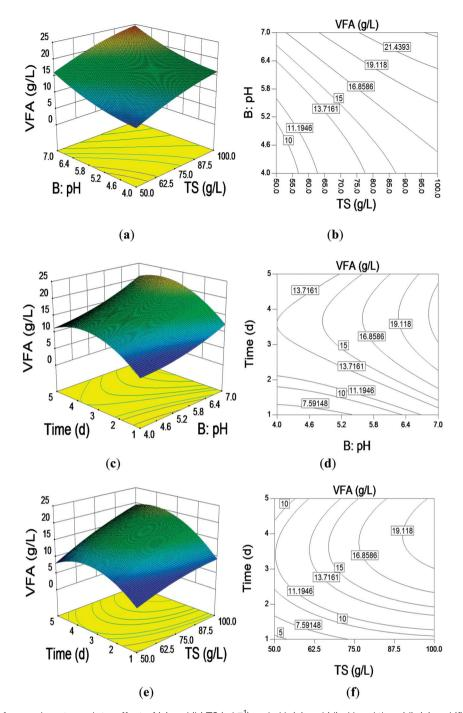
Fig. 1 3D response surface and contour plots: effect of (a) and (b) TS (g  $L^{-1}$ ) and pH; (c) and (d) pH and time (d); (e) and (f) pH TS (g  $L^{-1}$ ); and time (d).
