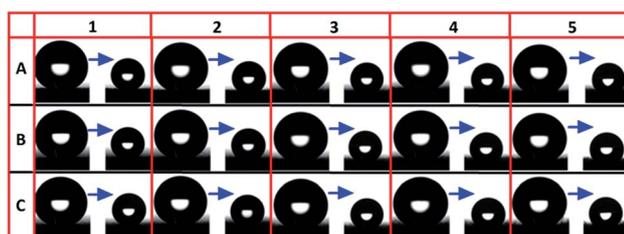
Fig. 3 Evaporation test of flocking samples, showing the water droplet change from the beginning to 60 min thereafter.
