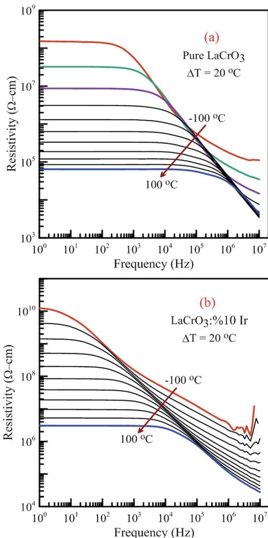
Fig. 15 Frequency dependence of the resistivity of both samples in the temperature range from  $-100\text{ }^{\circ}\text{C}$  to  $100\text{ }^{\circ}\text{C}$  with steps of  $20\text{ }^{\circ}\text{C}$ , (a) pure  $\text{LaCrO}_3$  and (b)  $\text{LaCrO}_3:10\%\text{Ir}$ .
