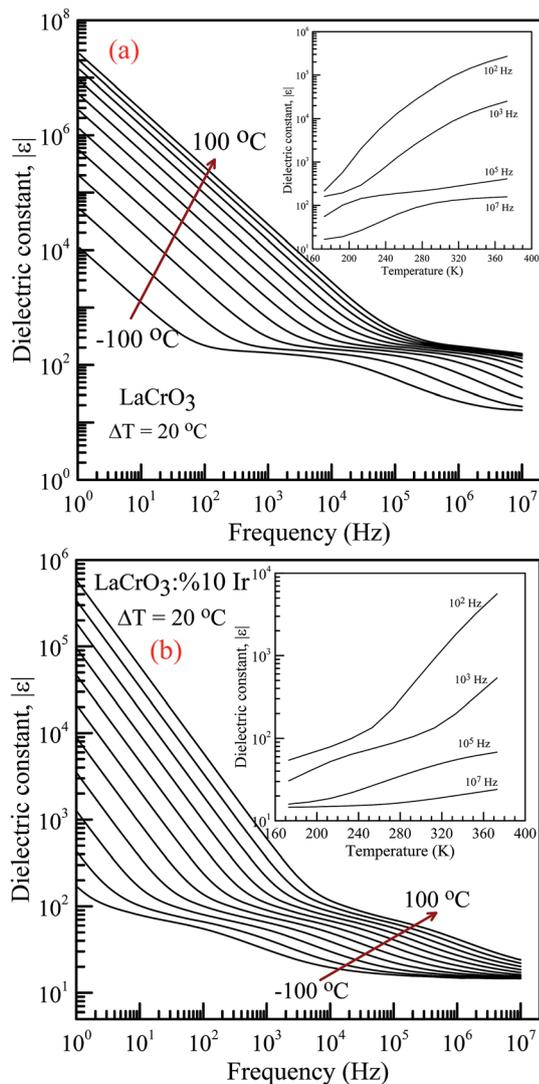
Fig. 4 Frequency dependence of the dielectric constant  $|\epsilon|$  in the temperature range from  $-100\text{ }^{\circ}\text{C}$  to  $100\text{ }^{\circ}\text{C}$  with steps of  $20\text{ }^{\circ}\text{C}$ , (a) pure  $\text{LaCrO}_3$  and (b)  $\text{LaCr}_{0.90}\text{Ir}_{0.10}\text{O}_3$ . Inset figures show  $|\epsilon|$  vs.  $T$  at  $10^2$ ,  $10^3$ ,  $10^5$  and  $10^7$  Hz.
