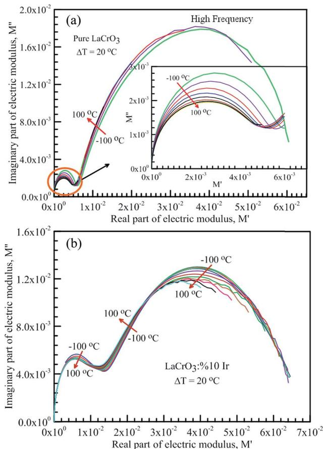
Fig. 8 Frequency dependent-electrical modulus plane plots, the imaginary  $M''$  versus real  $M'$  in the temperature range from  $-100^\circ\text{C}$  to  $100^\circ\text{C}$  with steps of  $20^\circ\text{C}$ , (a) pure  $\text{LaCrO}_3$ , inset: low frequency data of the complex electric modulus plane plot of the pure LCO sample, and (b)  $\text{LaCr}_{0.90}\text{Ir}_{0.10}\text{O}_3$  sample.
