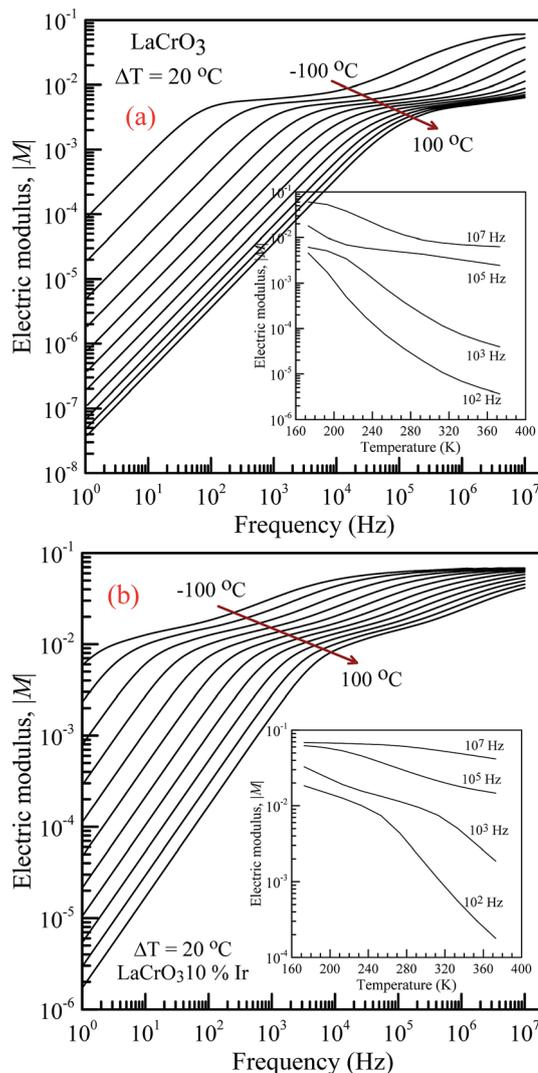
Fig. 5 Frequency dependence of the electrical modulus of both samples in the temperature range from  $-100\text{ }^{\circ}\text{C}$  to  $100\text{ }^{\circ}\text{C}$  with steps of  $20\text{ }^{\circ}\text{C}$ , (a) pure  $\text{LaCrO}_3$  and (b)  $\text{LaCr}_{0.90}\text{Ir}_{0.10}\text{O}_3$ . Inset figures represent  $|M|$  vs.  $T$  at  $10^2$ ,  $10^3$ ,  $10^5$  and  $10^7$  Hz.
