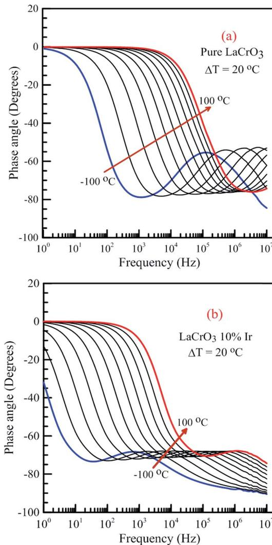
Fig. 14 Frequency dependence of the phase angle of both samples in the temperature range from  $-100\text{ }^{\circ}\text{C}$  to  $100\text{ }^{\circ}\text{C}$  with steps of  $20\text{ }^{\circ}\text{C}$ , (a) pure  $\text{LaCrO}_3$  and (b)  $\text{LaCr}_{0.90}\text{Ir}_{0.10}\text{O}_3$  samples.
