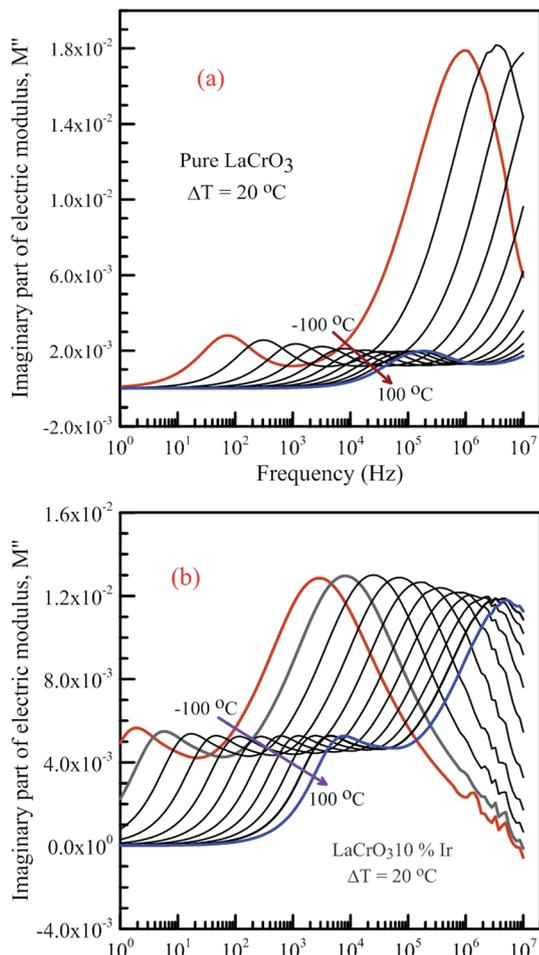
Fig. 7 Frequency dependence plots of the imaginary part of electrical modulus,  $M''$  in the temperature range from  $-100^\circ\text{C}$  to  $100^\circ\text{C}$  with steps of  $20^\circ\text{C}$ , (a) pure  $\text{LaCrO}_3$  and (b)  $\text{LaCr}_{0.90}\text{Ir}_{0.10}\text{O}_3$ .
