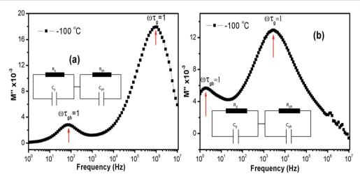
Fig. 11 The M'' vs. frequency behaviour for LCO and Ir doped LCO just at -100 °C and the relaxation points ( $\omega_{\text{max}}\tau=1$ ). Inset figures show equivalent circuit for each compounds.
