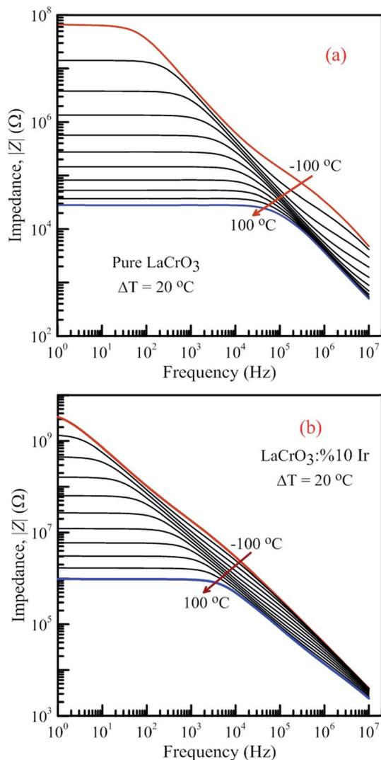
Fig. 13 Frequency dependence of the impedance of both samples in the temperature range from  $-100\text{ }^{\circ}\text{C}$  to  $100\text{ }^{\circ}\text{C}$  with steps of  $20\text{ }^{\circ}\text{C}$ , (a) pure  $\text{LaCrO}_3$  and (b)  $\text{LaCr}_{0.90}\text{Ir}_{0.10}\text{O}_3$ .
