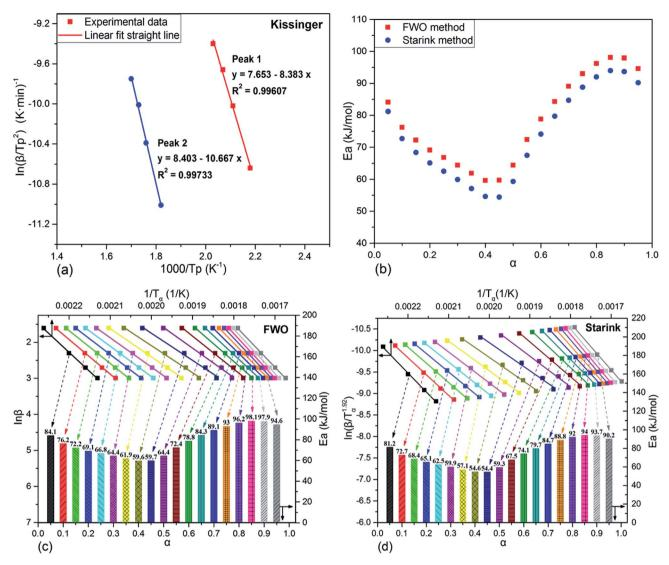
Fig. 6 Activation energy analyses of TGDDM/DICY system under different methods ((a) Kissinger plots of the two cure processes; (b) variation of activation energy versus fractional conversion from FWO method and Starink method; (c) FWO plots at different fractional conversions; (d) Starink plots at different fractional conversions).
