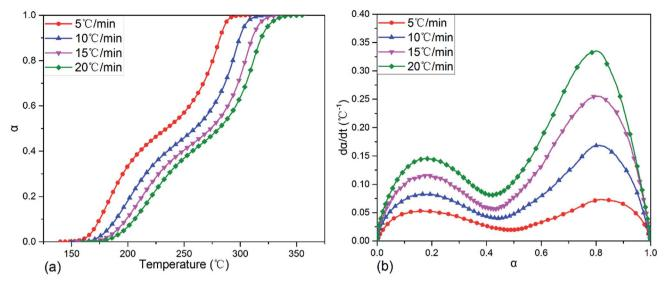
Fig. 5 Plots of fractional conversion vs. temperature (a) and reaction rate  $d\alpha/dt$  vs. fractional conversion (b) for TGDDM/DICY system at different heating rates
